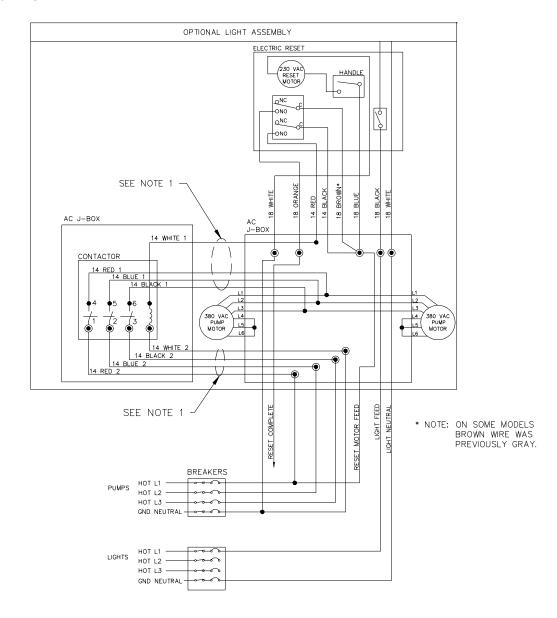
NOTE 1: WIRES FROM MAIN AC J-BOX TO AUXILIARY CONTACTOR J-BOX ARE LABELED "1" OR "2" AS INDICATED ON BOTH ENDS
