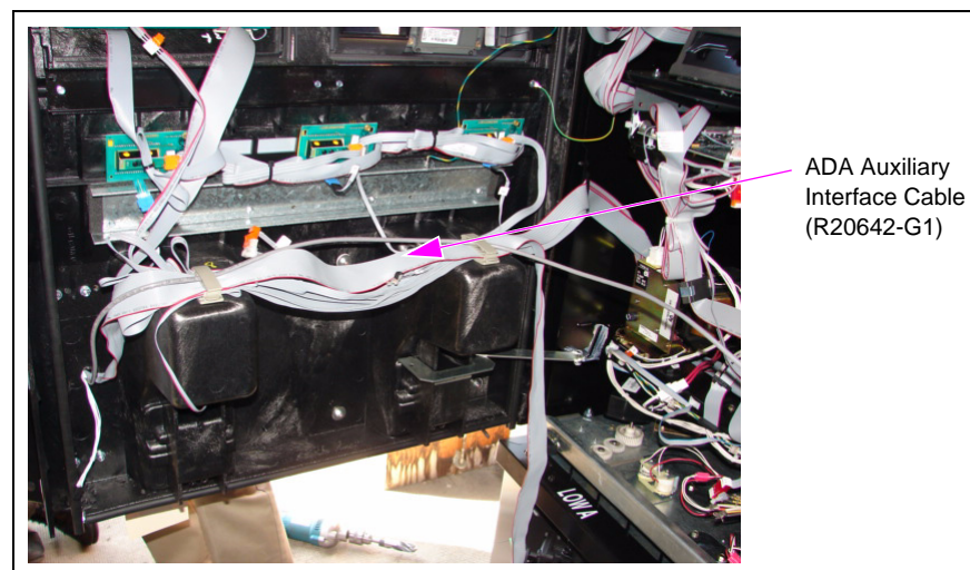
Figure 17: Clamping the ADA Auxiliary Interface Cable (R20642-G1)
