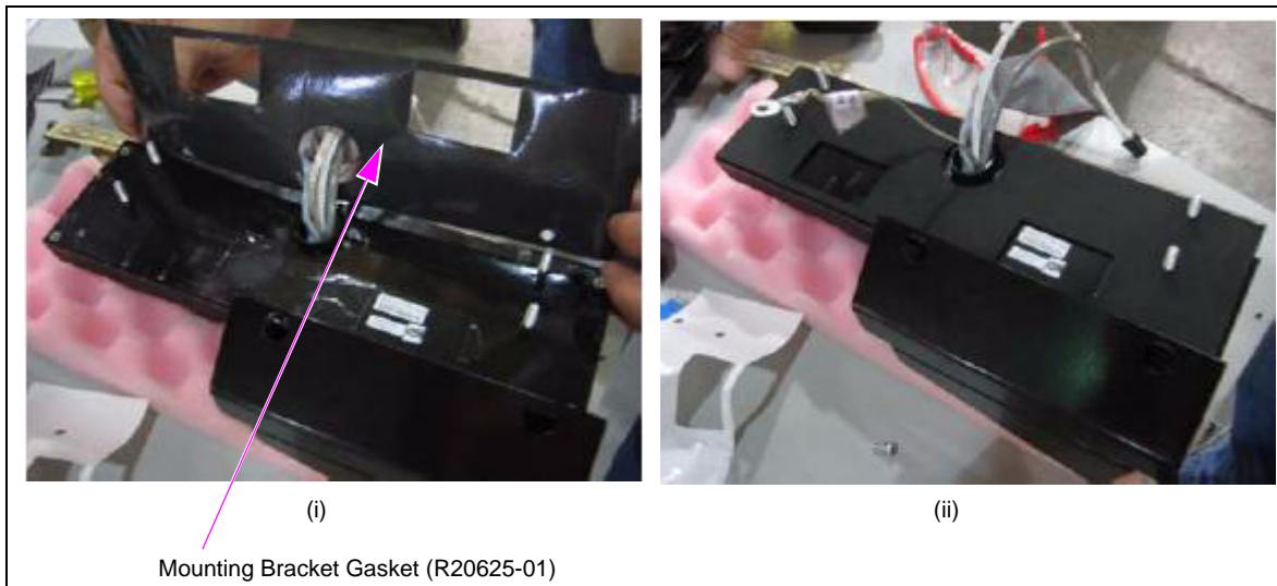
Figure 37: Installing the Mounting Bracket Gasket (R20625-01)
