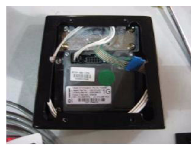
Figure 30: Replacing the ADA Gasket (M09840B001)
