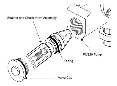
For K35220, remove strainer from check valve. Install new strainer as shown below.
