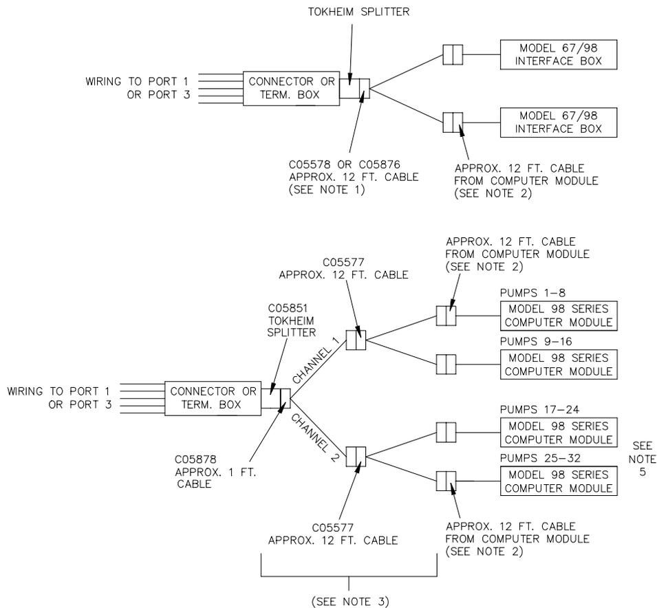
1. Use a C05578 cable for connection to a single 67 or 98 Interface box. Use a C05876 cable for connection to two 67 or 98 Interface boxes. Both cables include the Tokheim Splitter.
