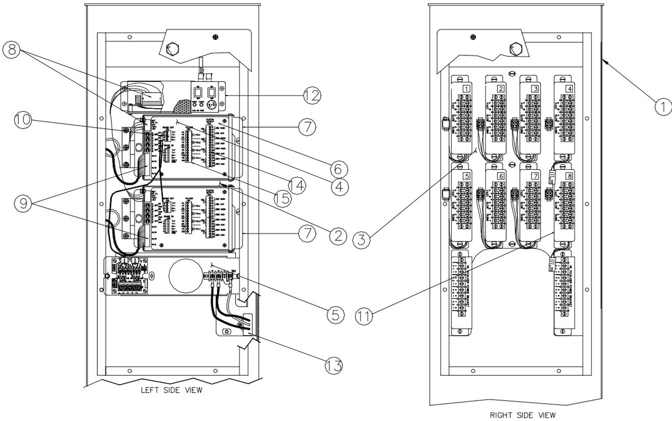
**C07558 Standalone Pump Control Unit, 8 Hose Fleet Mechanical (Fleet)**
