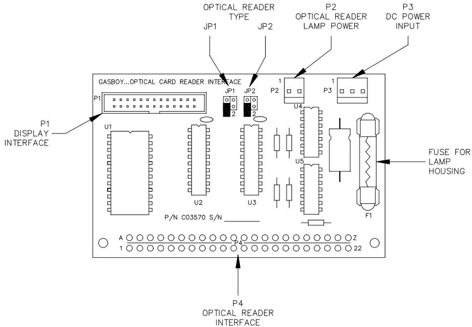
There are two versions of this board: Densitron and Beckman. While they look identical, they are not interchangeable. On the Densitron board, the dashed line is below the P1 connector; on the Beckman, the dashed line is above the P1 connector.
