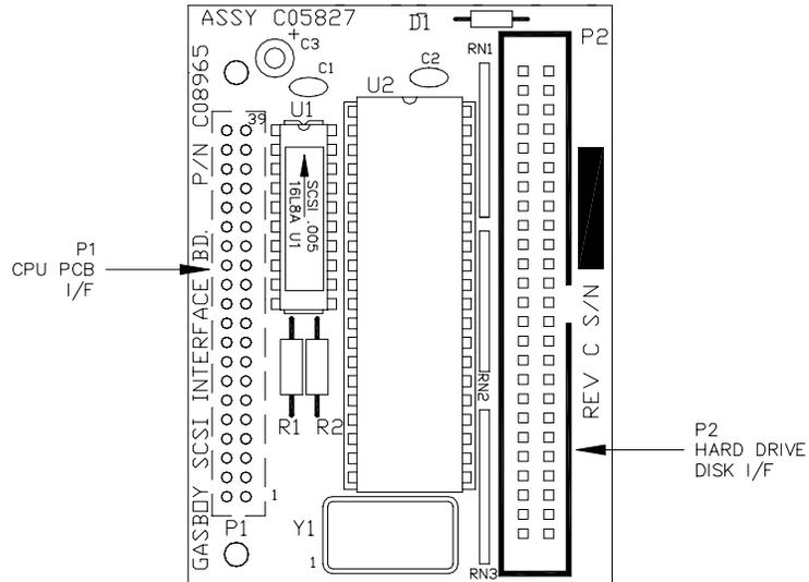
Rev. D or greater SCSI interface board requires version 1.0K or above. DSITE V3.2C or above is required to work with updated SCSI interface board (C05827); newer hard drives will require DSite V3.3B or above.
