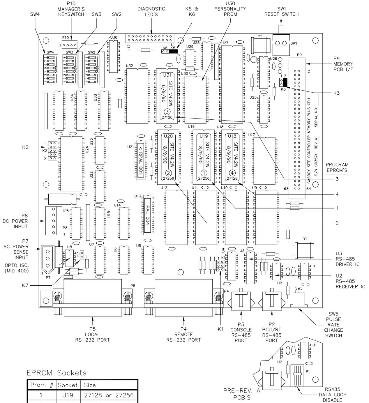
Layout - Site Controller I CPU - 512K PCB (C05820)
