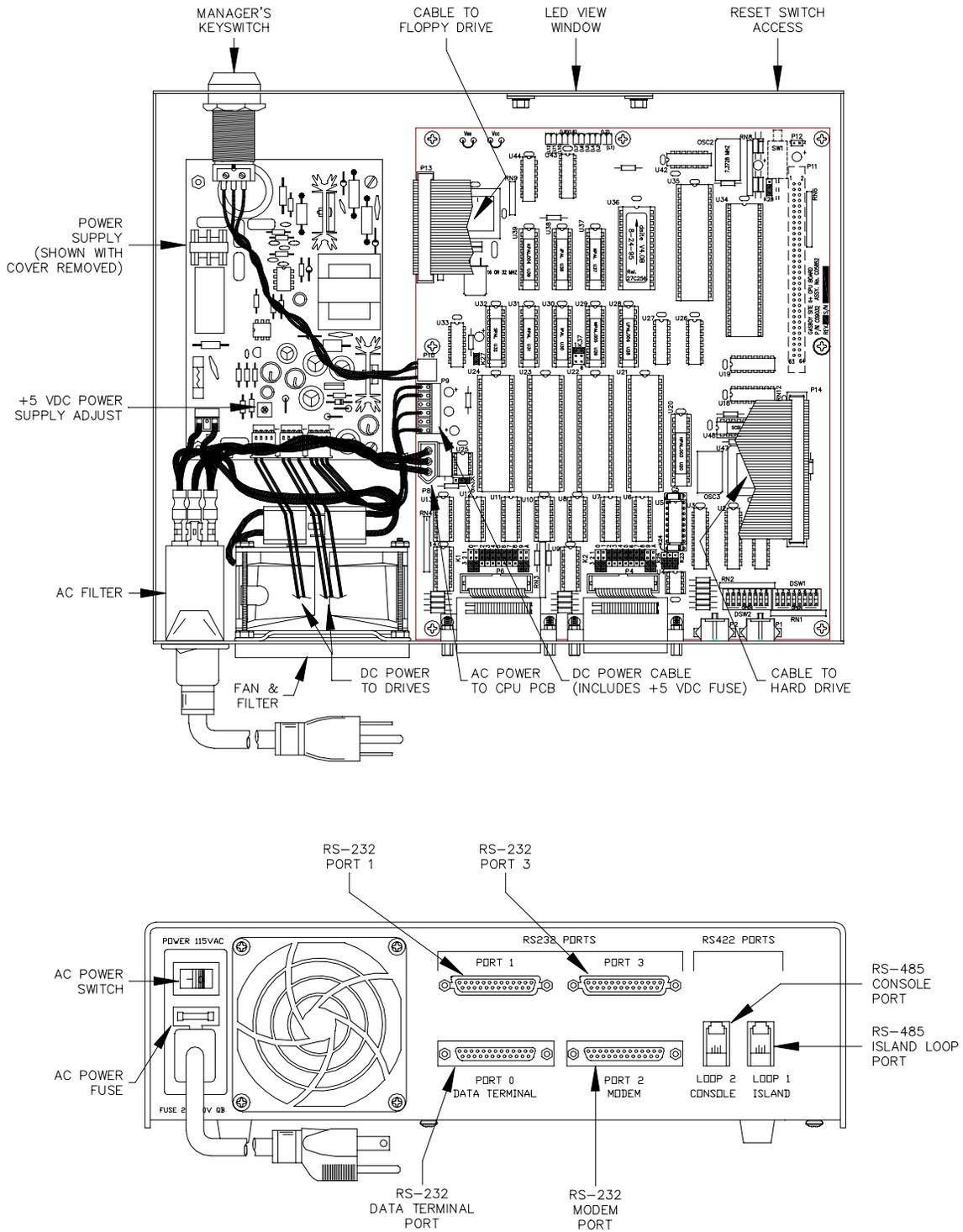
**3-1/2" Disk Drive Model (Single Drive, C05574; Dual Drive, C05575)**
