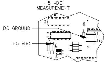
For C05857 board: Measure the +5VDC between test points TP1 (5V) and TP2 (Gnd). The voltage should be +5.00 to +5.10 VDC. If the voltage does not fall within this range, adjustment is necessary. Follow the steps below to adjust the supply. If the voltage is within tolerance, skip to Step 14.
