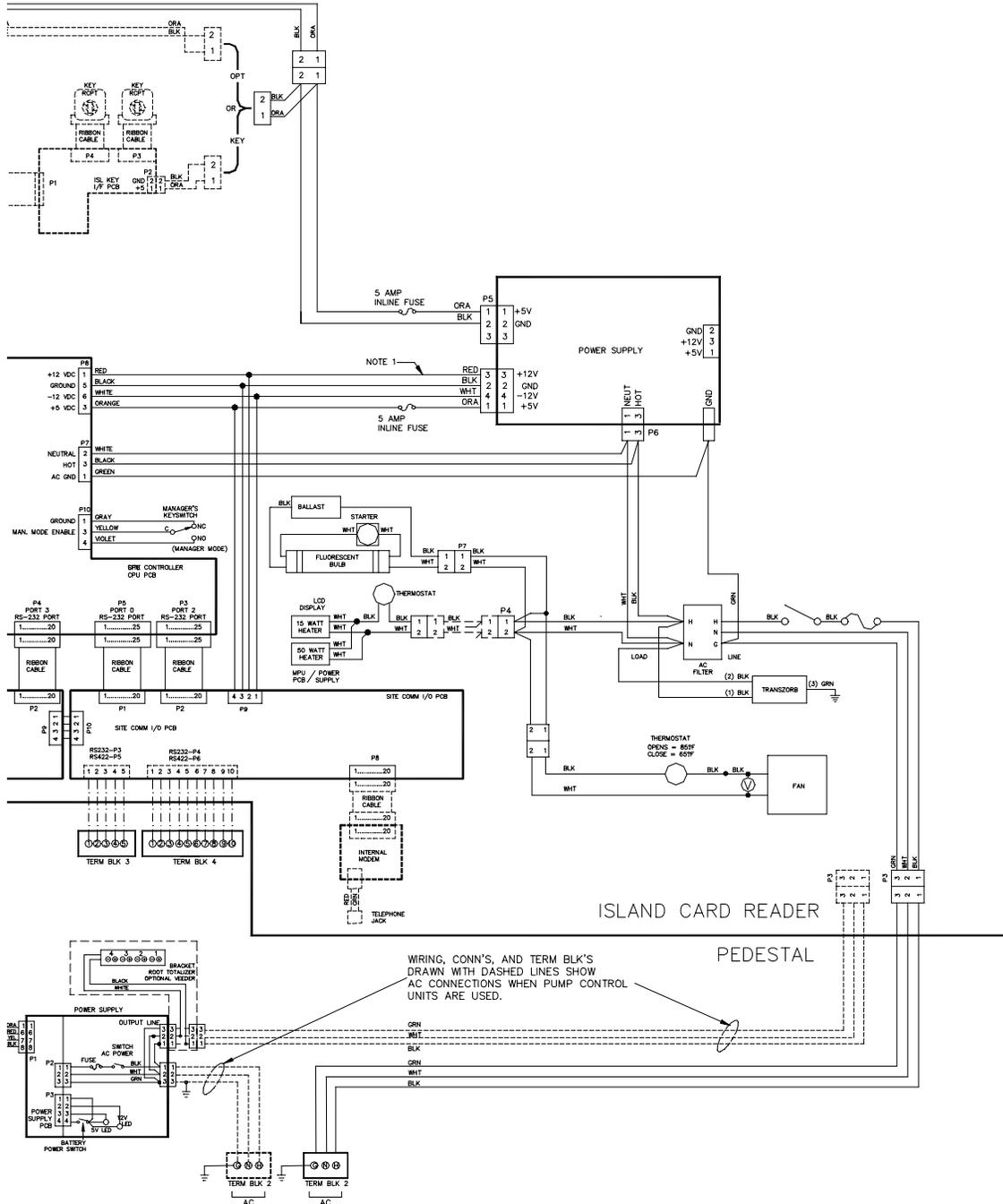
WIRING, CONN'S, AND TERM BLK'S DRAWN WITH DASHED LINES SHOW AC CONNECTIONS WHEN PUMP CONTROL UNITS ARE USED.
