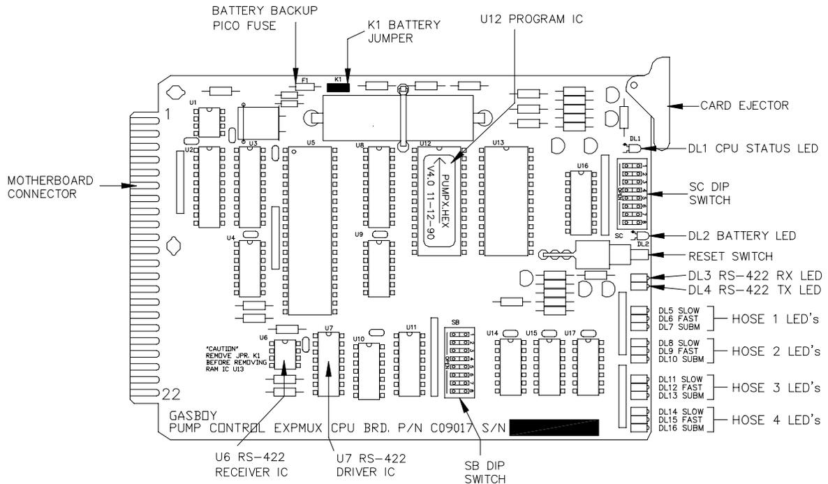
This drawing shows the EXPMUX CPU PCB orientation in the pump control unit.
