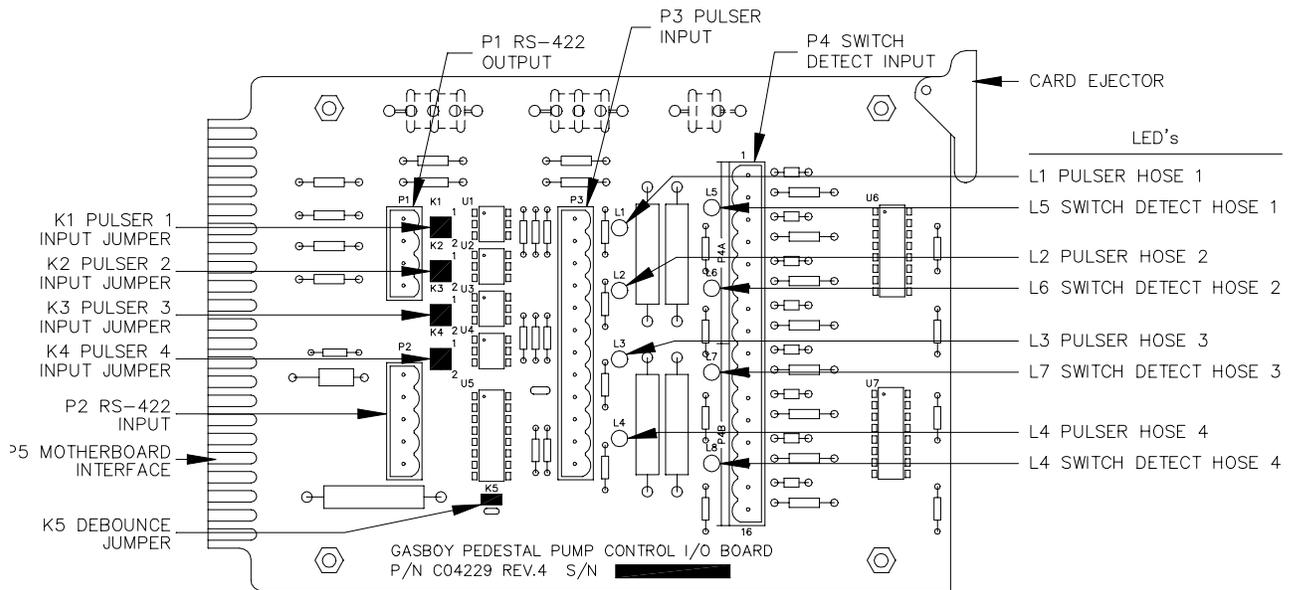
This drawing shows the Pump Control I/O PCB orientation in the pump control unit.
