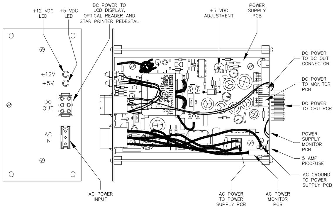
**NOTE:** Power One supply is shown. Location of +5VDC adjuster may vary depending on supply. See Section 2 or 3 for illustration of power supply types and adjuster locations.
