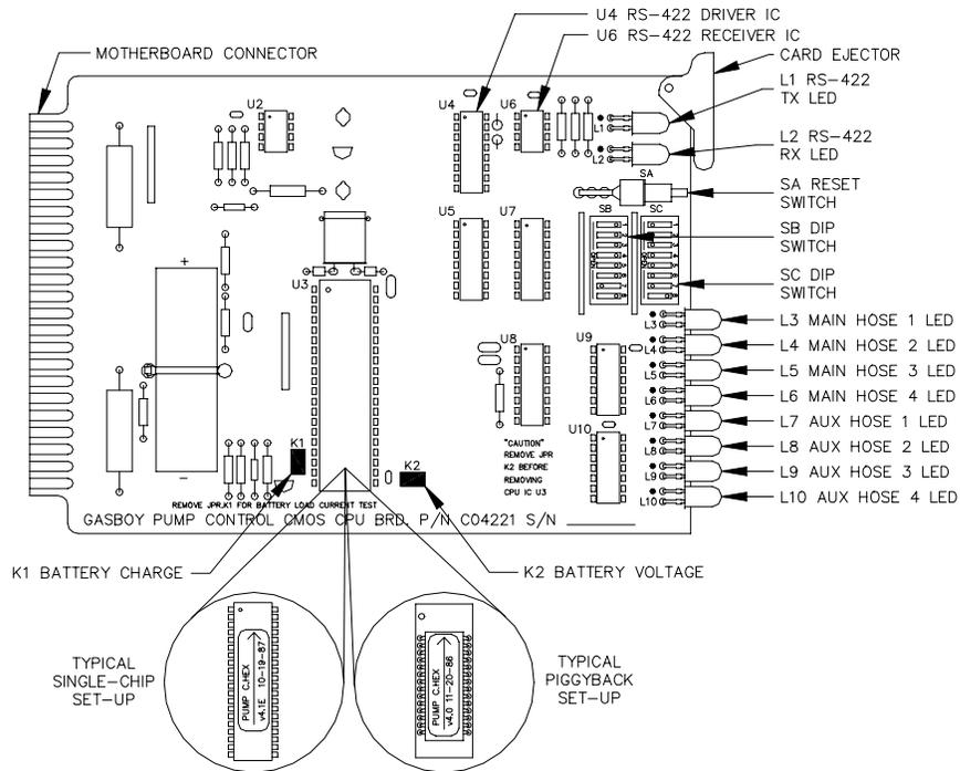
This drawing shows the CMOS CPU PCB orientation in the pump control unit.
