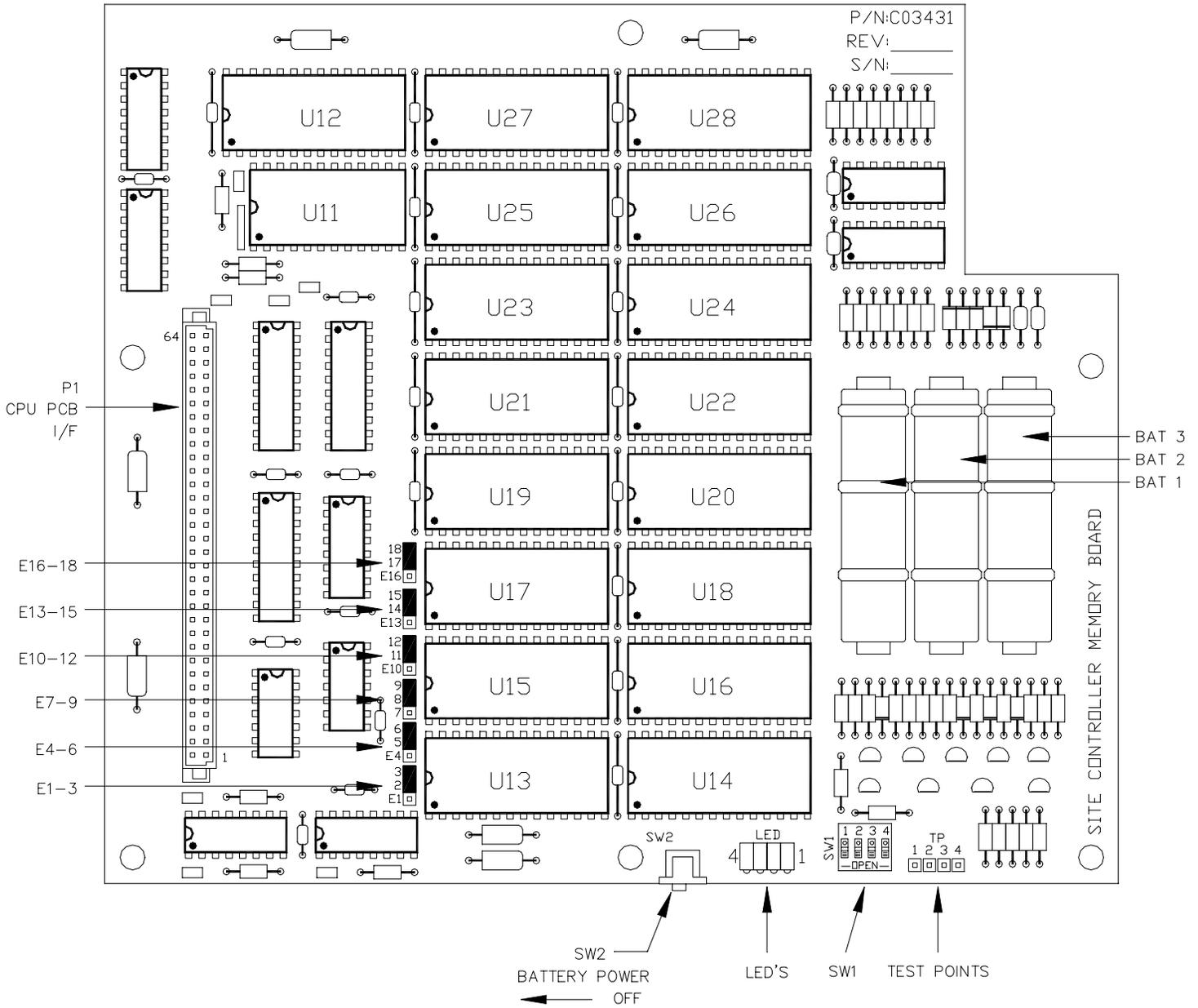
**Site Controller II Memory PCB Layout (C02117: U14 - 31 contains 8K chips)
