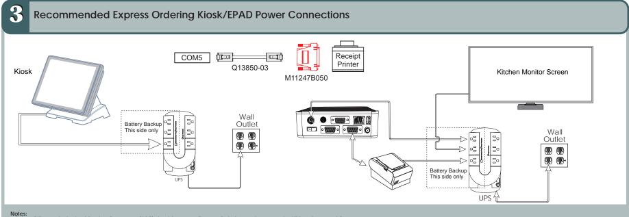
Notes: • Only a Gilbarco Authorized Service Contractor (ASC) should connect Express Ordering equipment to the UPS and turn on AC power • Connect only Express Ordering equipment to the UPS. Do not power any other equipment from the UPS.
