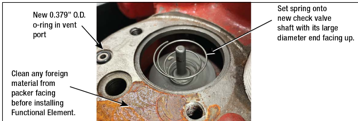
Figure 10. Installing Check Valve And Spring In Packer
