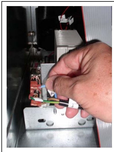
Figure 24: Connecting UPM AC Power Cable to AC Line Filter Power Supply Cable
