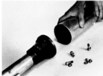
2. Rock unit while pulling away from discharge head until free.
