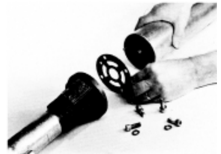
3. TO RE-ASSEMBLE: Replace gasket, align dowel pin, draw in place with cap screws.
