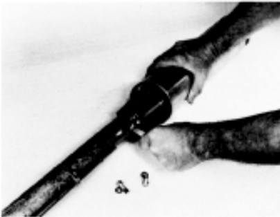
1. Remove the four screws holding motor to the head casting.
