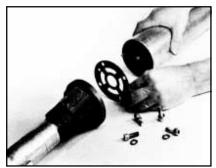
TO RE-ASSEMBLE: Replace gasket, align dowel pin, draw in place with cap screws.
