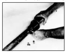
Remove the four screws holding motor to the head casting.
