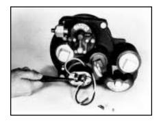
2. Remove retaining clip. Pull quickconnectors.
