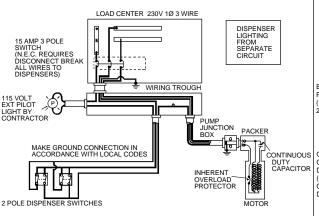
Suggested wiring diagram WITHOUT optional control box. Combination of 1 pole dispenser switches or external pilot light requires special instructions - consult factory.
