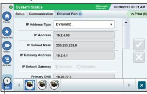
Touch **Actions>Help** from this screen for setup assistance. Ethernet ports 2 and 3 are an optional feature.
