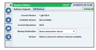
Insert your thumbdrive (minimum 4 GB) in a USB port and touch the down arrow in the Backup Destination field to select the thumbdrive, then follow the on-screen instructions to backup TLS4 data.
