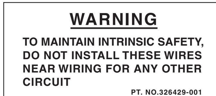
**Figure 2.** Dispenser Control Interface WARNING Label
