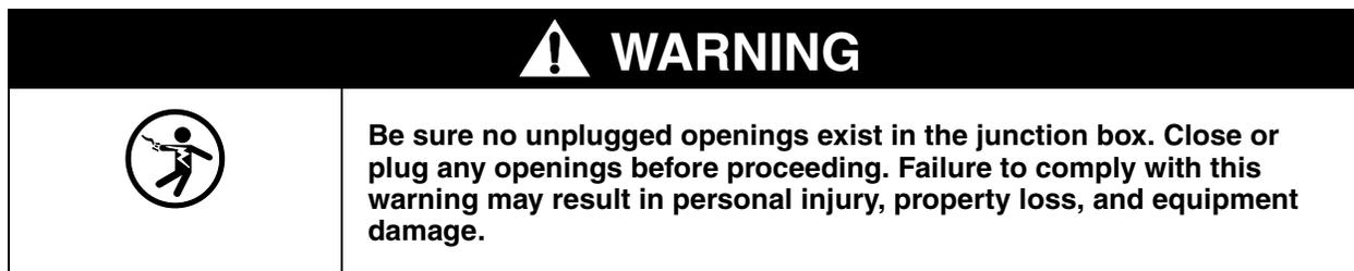
2. Place the cover on the junction box and ensure that all cover screws are replaced and tight.
