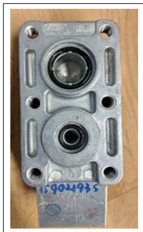
Figure 26: O-ring on Vapor Recovery Port
