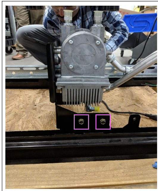
Figure 6: Motor Attached to “B” side of Encore Frame
