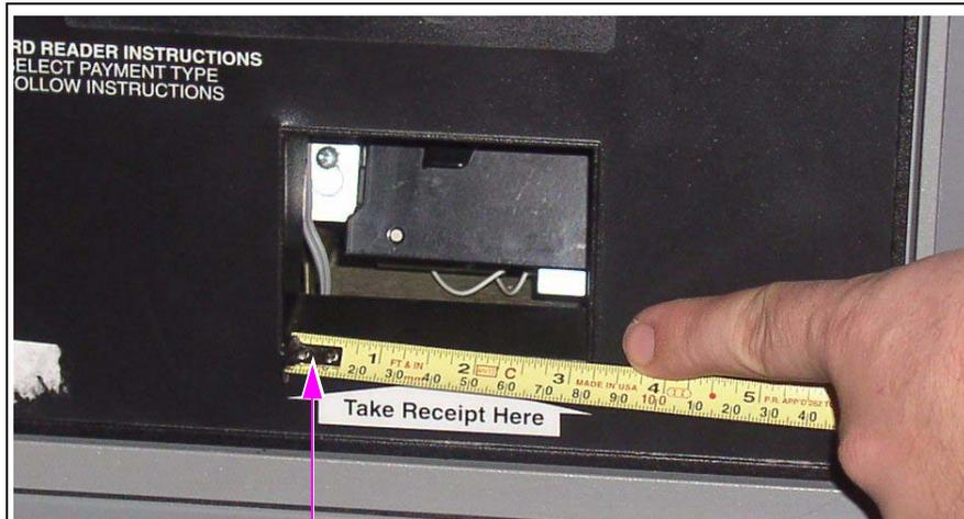
Printer Chute Opening Dimension - Models Built Prior to 1995 (3.25")
