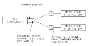
Part number C06694 includes the Tokheim Splitter, the C05878 cable, and two C05577 cables; it connects the Site Controller II to three or more 98 boxes.
