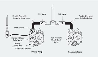
Manifolded systems provide up to 2X the flow rate and improved uptime. Manifolded systems can be configured in sumps 42" in diameter or greater.
