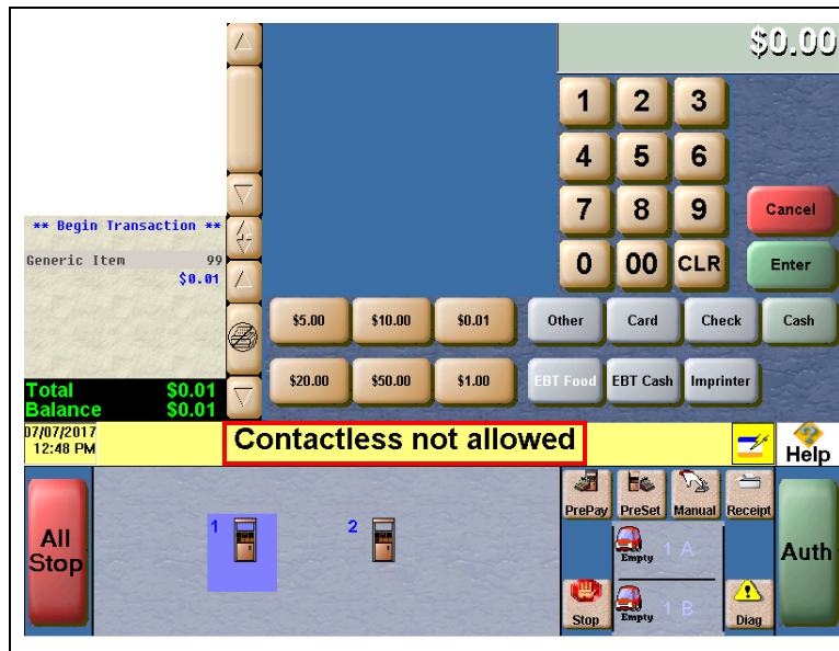
Figure 15: CWS Message when tapping a Contactless EMV Card
