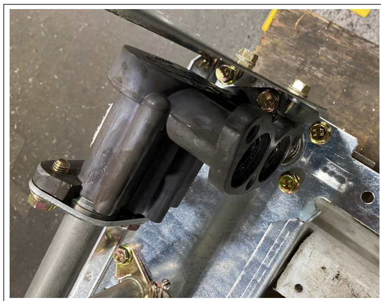
Figure 34: Angle Casting with Hard Anodizing (Dark Finish) for E85 Compatibility
