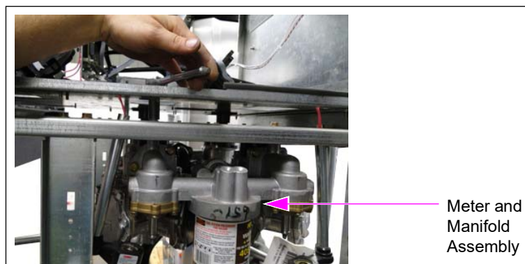
Figure 8: Removing Screws Holding Meter and Manifold Assembly
