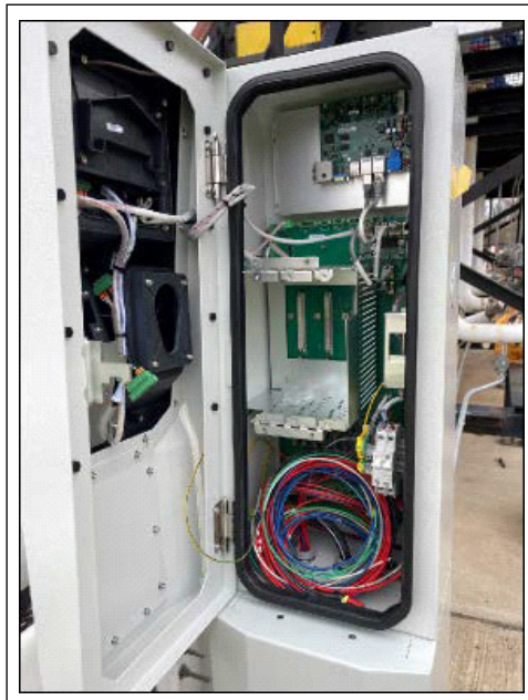
Figure 4-1: Inside Door Before Installation
