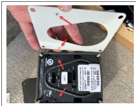
Figure 4-3: PIN Pad Back Plate
