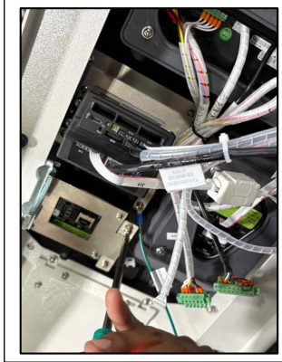
Figure 4-16: Securing Contactless Reader Support Bracket Screws
