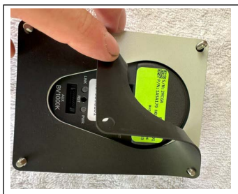
Figure 4-4: Mount the PIN Pad Plate Rubber Gasket
