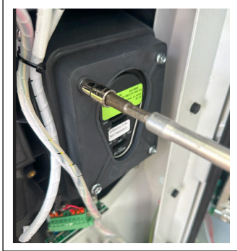
Figure 4-5: Secure the PIN Pad with the Nuts
