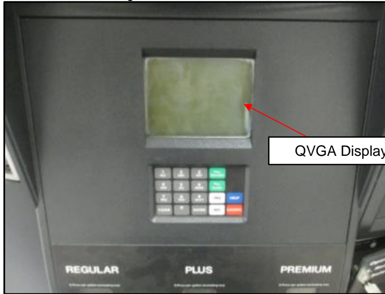
Front side of QVGA Panel showing display glass
