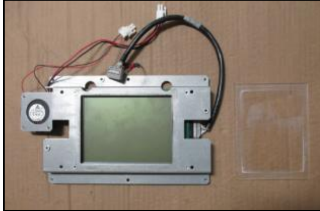
Backside of QVGA retainer bracket and customer LCD display
