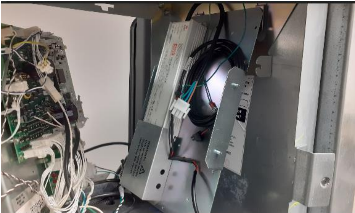
PSU Assembly (EZ0853) placed inside dispenser. Side B Vista 4V Narrow shown.
