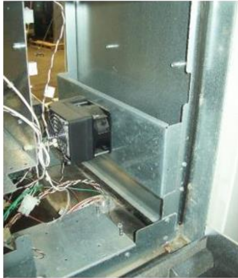
Heater mounted at lower side. Needs to be relocated to fit Power Supply Brackets.
