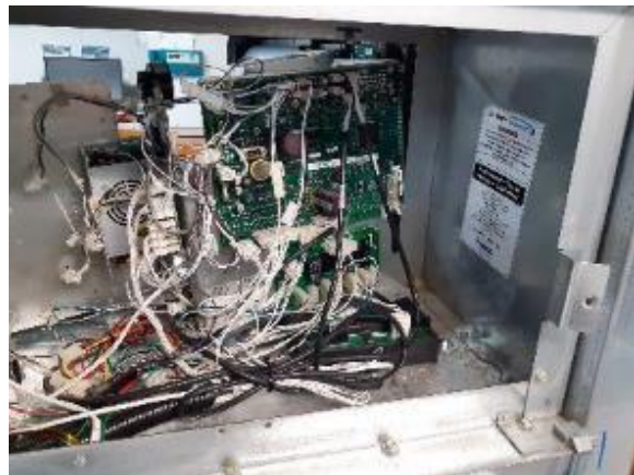
Carefully move panel diagonally. Side A Vista 4V Narrow shown.
