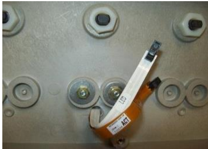
Fuel Grade Selector Button with two ribbon cables. The LED Plugs above the button are not removed with this type of Selector, as it has built in LEDs.
