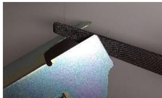
Cut off the tabs and file off sharp edges.
