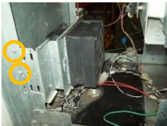
Remove Screws, Side A
