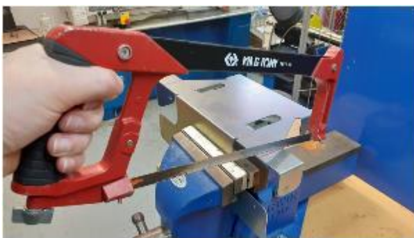
Cut off the tabs and file off sharp edges.
