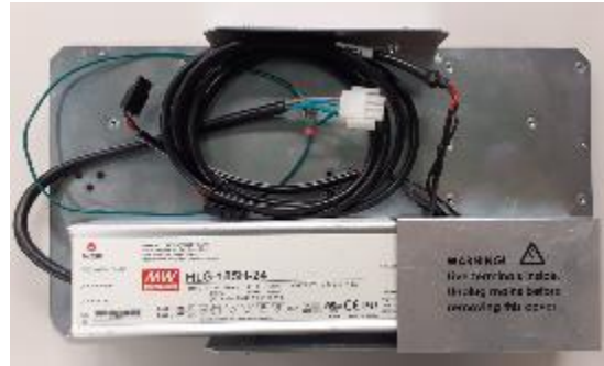
Side B: PSU Assembly (EZ0853) with cables
