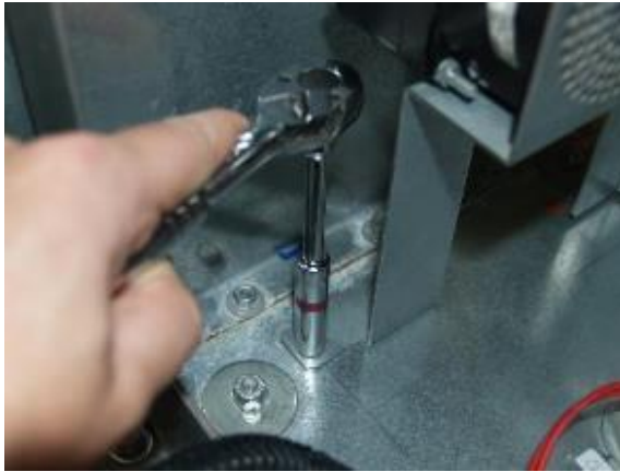
Undo Electronics Panel feet mounting nuts. Vista 4V Wide shown.
