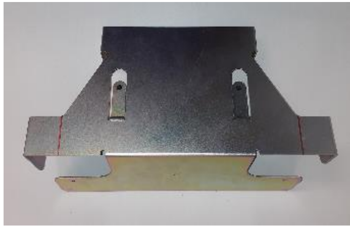
Mark two cut-lines on the tabs
