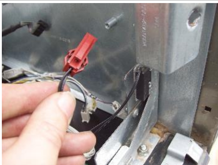
If fitted, disconnect and label the cable to the Security Reed Switch sensor. It will be reconnected later.
