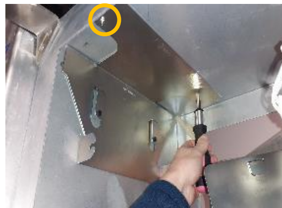
Attach using the two lid mounting nuts. Side A Vista 4V Narrow shown.
