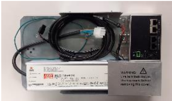
Side A: PSU Assembly (EZ0853) with cables and InvencoLink
