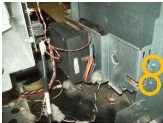
Remove Screws, Side B
