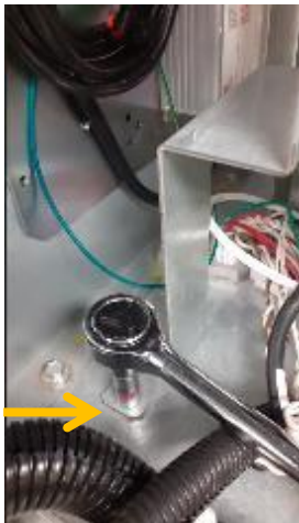
Tighten Mounting Nuts. Vista 4V Narrow shown.
