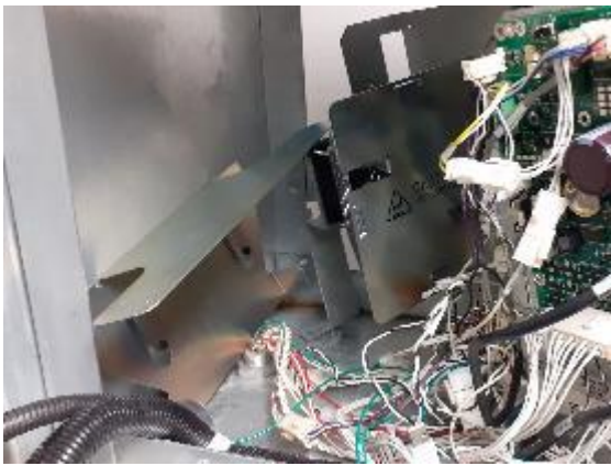
Place PSU Assembly inside dispenser. Side A Vista 4V Narrow shown.
