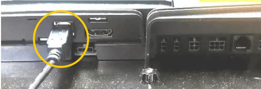
22. If this installation has an ADA keypad (found beside the Contactless module on the Contactless RFK Panel), insert the ADA connection cable (shown bottom left) from that module into the Display RFK Panel ADA socket.
