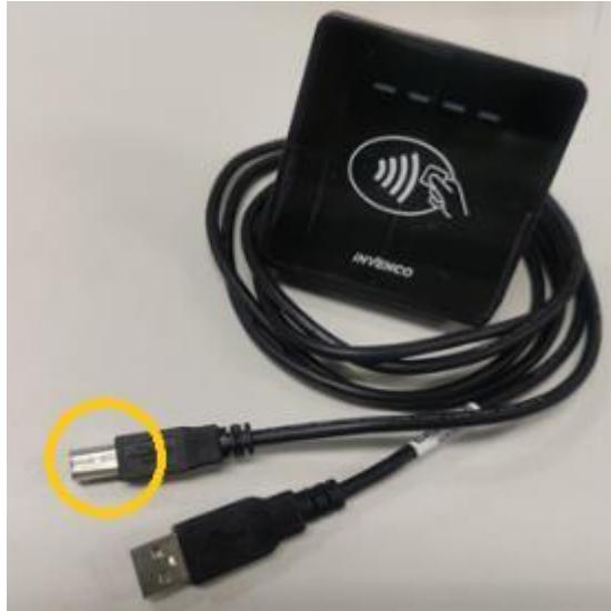
Insert the Type B connector into the “APC-USB” socket on the display (SDC) module.
