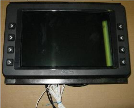
Contactless RFK Panel with cables (RP00035-XX):
