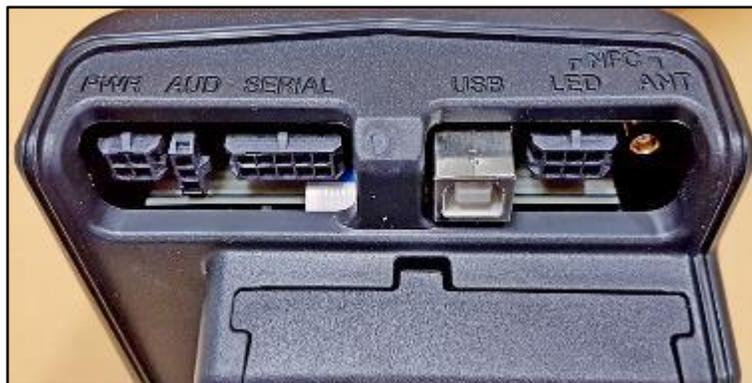
All of the cables on the Display RFK Panel are pre-installed and loomed, and each connector is different so there can be no wrong connections made.
