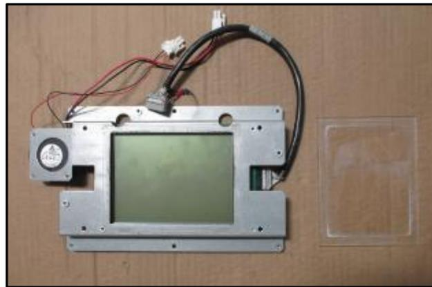
QVGA LCD display, retainer, and glass after removal
