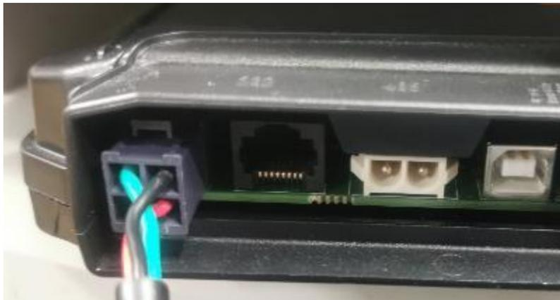
26. Locate the ETHERNET connector on the Display RFK Panel (also use picture in Step 24).
