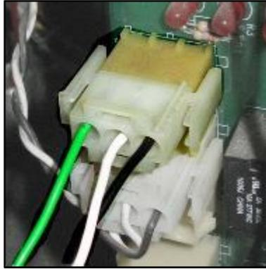
5. Connect the Plug removed in Step 3 into the Socket on the double-connector end of the EK0137 AC Mains cable:
