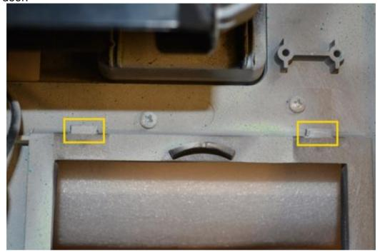
b. Install the provided screws MS0245 (006-8611475) in the lower section of the printer assembly and attach to the Helix G7 or G7 15 inch panel.
