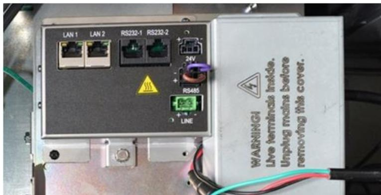
3. Install the Helix PSU Assembly with the Dispenser InvencoLink facing out towards you on the dispenser side opposite the pump controller board. Place the full Helix PSU Assembly into the dispenser cavity in the farthest back plastic bracket slots located in the center of the dispenser.
