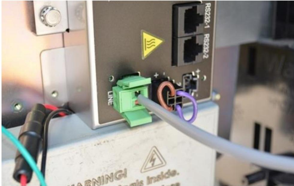
7. Connect the preinstalled PSU power cables to the previously routed Helix power adapter cables.
