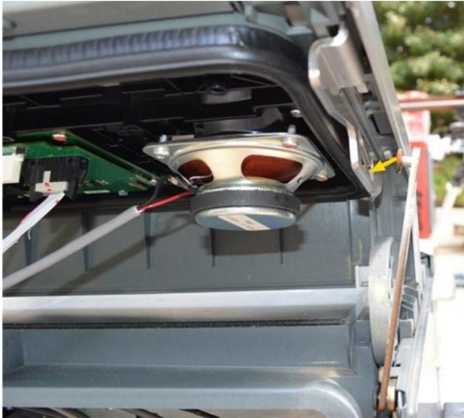
3. Check to verify that the dispenser does not have an existing intercom speaker. Visually identify to see if the intercom speaker is present on the upper plastic collar frame. If an intercom speaker is present, this installation guide does not cover installation in this dispenser. Close up the dispenser again and contact
