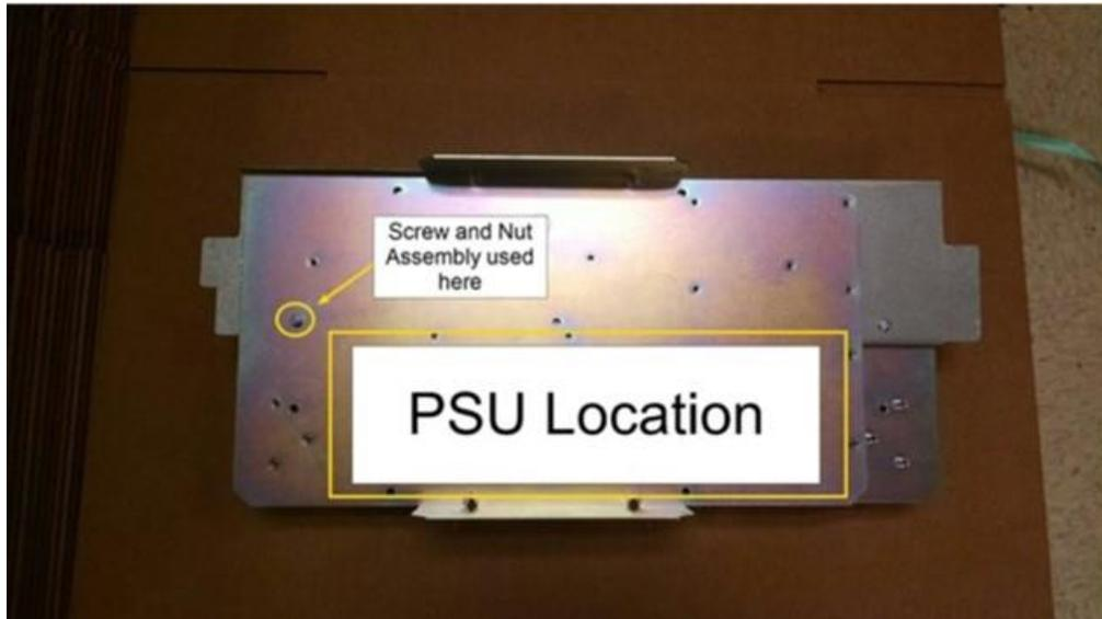
2. Install the Dispenser InvencoLink to one of the PSU brackets. Follow the InvencoLink Installation Instructions DCV-00465. Acquire the InvencoLink Retrofit Kit, UL Listed by Report Retrofit kit part number RF00033.
