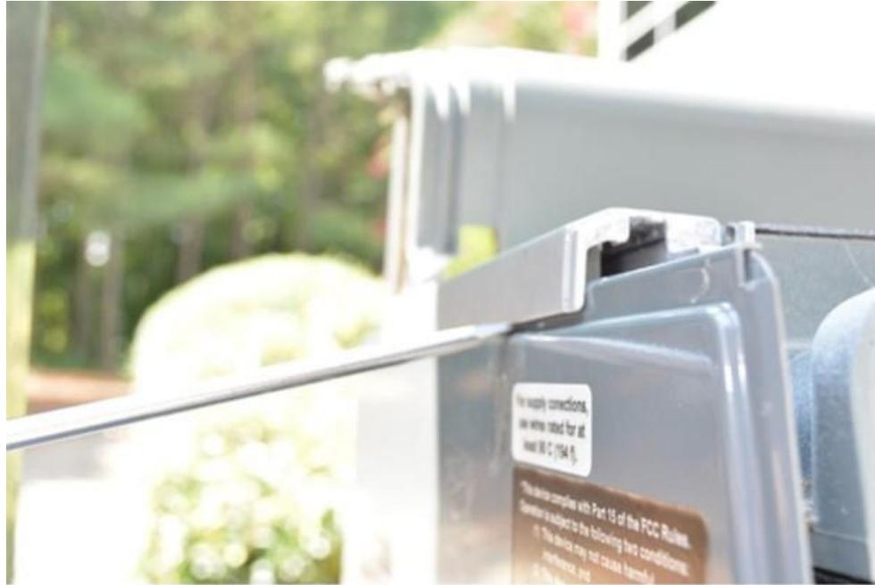
7. Verify the upper plastic collar frame on each side is raised and the prop rod is in place after both shoulders have been removed.
