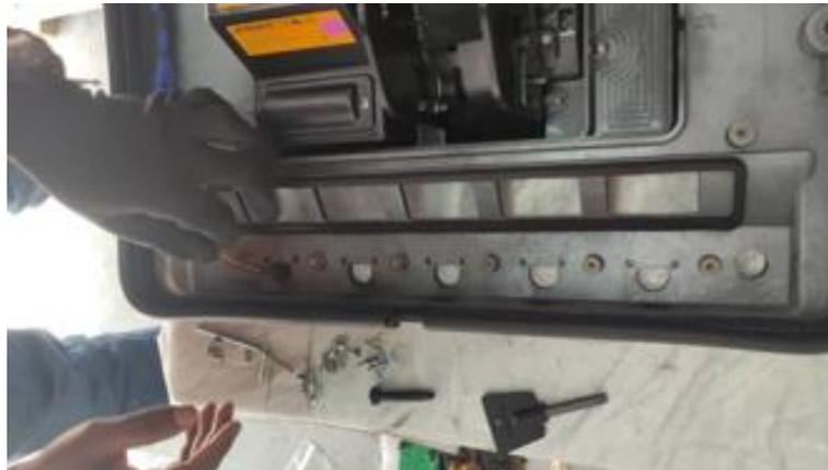
**Note:** Be sure to not to handle the ribbon cable roughly and also do not kink the ribbon cable between the back of the Push-To- Start Button assembly and the lower bezel door.
