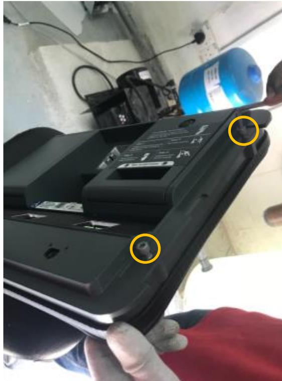
12. Lay the G6-300 Wayne Helix 2 lower Base Assembly (RP00084-XX or RP00091-XX) on its back and temporarily remove the metal bracket (4pcs of screw, M4 button head) and the glass cover using the Allen key sized 2.5mm. Retain all removed parts for later install.
