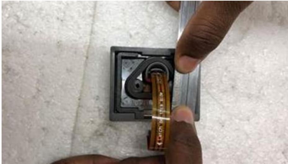
20. Install the push-to-start button paddles on the panel assembly by routing the ribbon cable through the “D shaped” opening in the new lower bezel. Ensure they are fitted in the same positions as they were in the Wayne panel.
