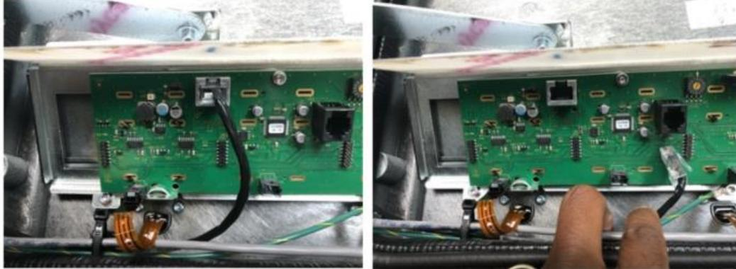
4. Remove M4 screw that secures the ground ring terminal to the bottom center hole using M3 Hex tool and discard the screw. Mark/Label Ground cable for subsequent installation.
