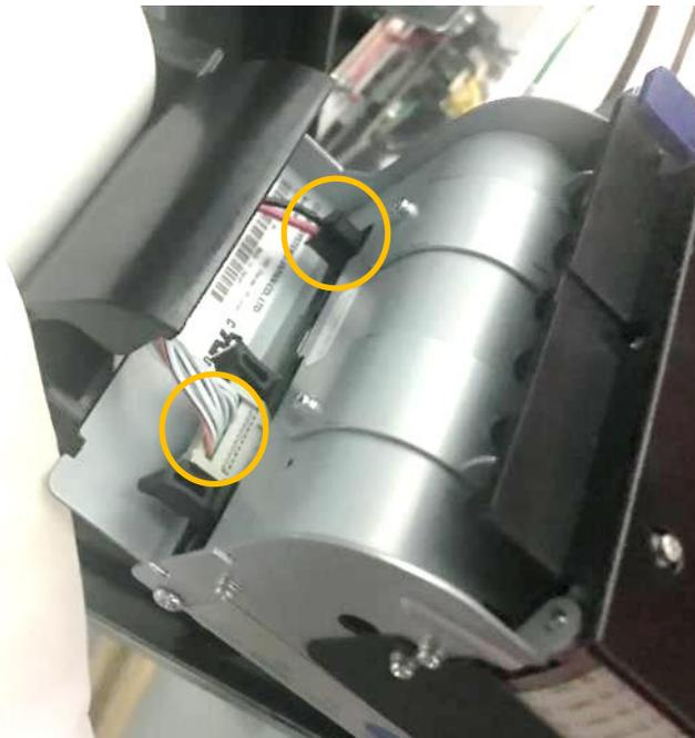
10. Cut the cable ties tied to the printer bracket
