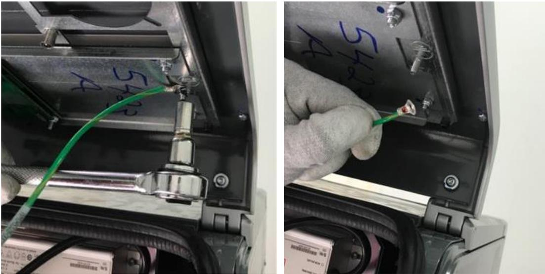
2. Remove all connections to the customer display and note the connection locations marked by green circles below that needs to be reconnected later.
