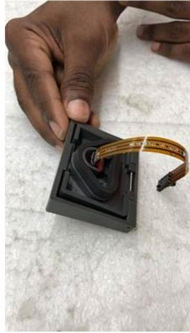
19. Using flat surface object such as metal ruler to apply pressure to the gasket on all corners.
