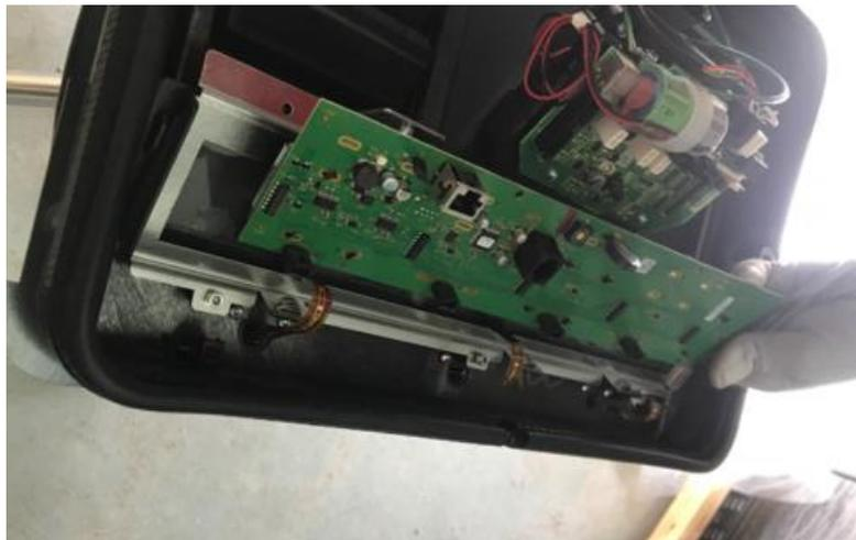
4. Remove the 2 remaining 3mm hex screws as shown in figure below. This will release the UPD bracket assembly from the lower bezel door. Retain screws for installation.
