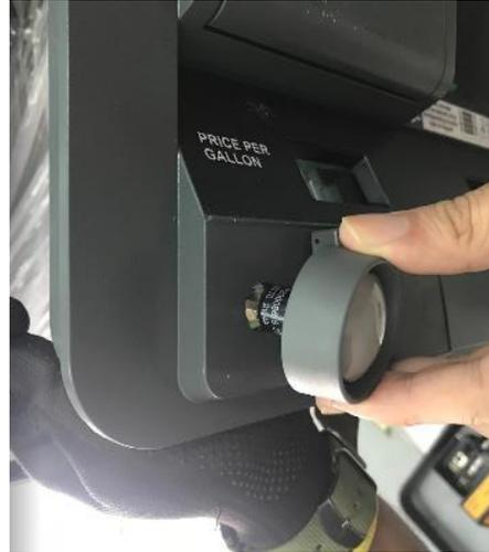
11. Remove and retain the 2 x Hinge screws using the M5 Hex tool.
