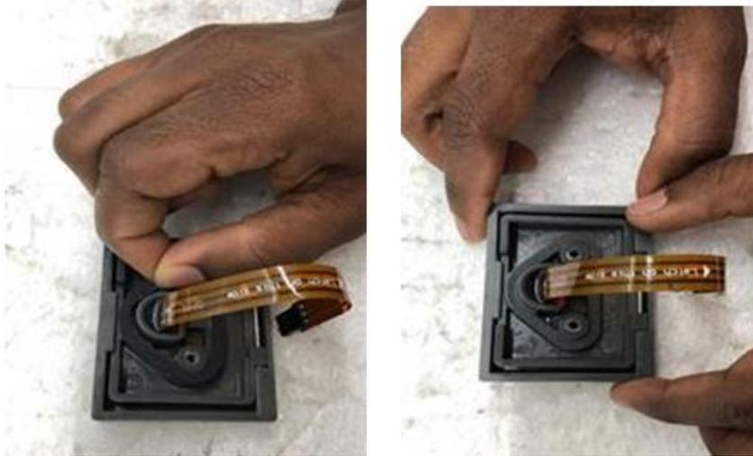
17. Peel off the release liner from MP1301 replacement gasket.
