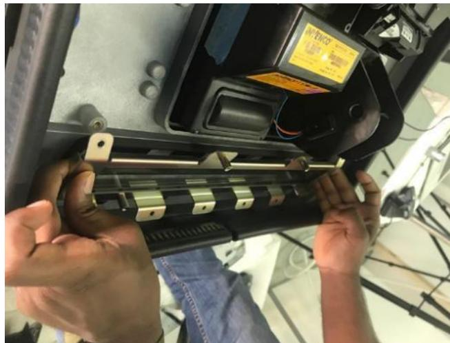
13. Install the lower bezel screw by using the Torx Key and screwing in from the front while threading the plastic lock washer on the back.
