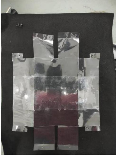
2. The insulation cover has pre-folded lines. Follow these lines in the same direction to fold. The cover is symmetrical so you can begin folding from any side. In the below images a metal bracket has been used to show the folds more clearly. However, the insulation cover can be folded in place with hands only.
