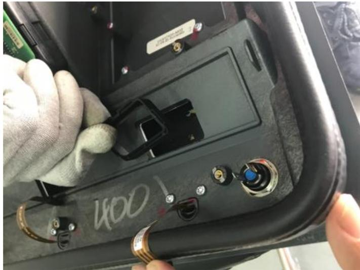
9. Remove lower bezel screw by using a flat edge object on the back/inside of the bezel and the Torx key used to open the lower bezel door on the front/outside of the bezel. Retain both components for re-installation.
