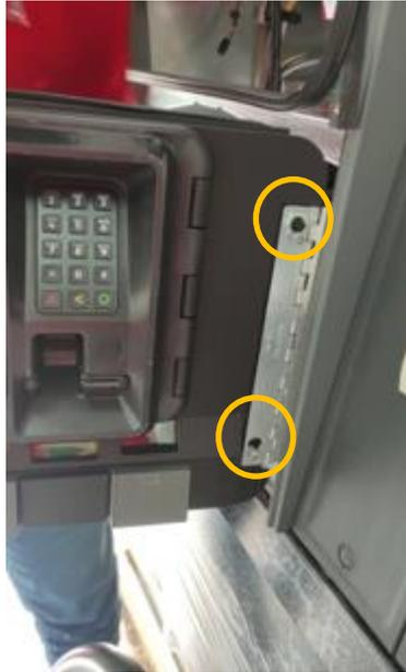
9. Attach previously labeled ground to bottom center hole in the UPD bracket on lower bezel by loosening the previously fitted screw using 2.5mm Hex tool.
