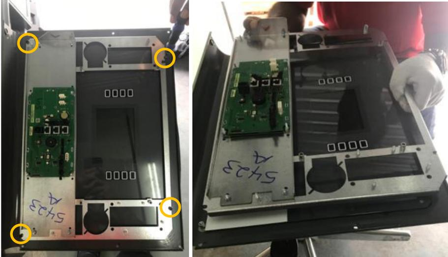
5. Assemble the remaining Bracket Assembly (that was removed in the above step) in the G6-300 Wayne Helix 2 Standard Upper Panel Assembly (MZ0298 or MZ0299) using the retained screws from the above step.
