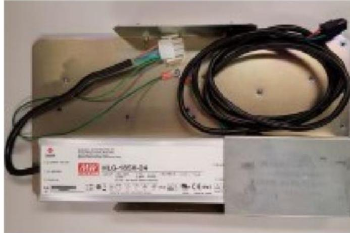
1. Attach both G6-300 Wayne Helix 2 Power Supply Assemblies (PSU) (EZ0704) to the Helix PSU Mounting Bracket (MP1275) using the provided nuts (MN0029) as shown in the pictures below.
