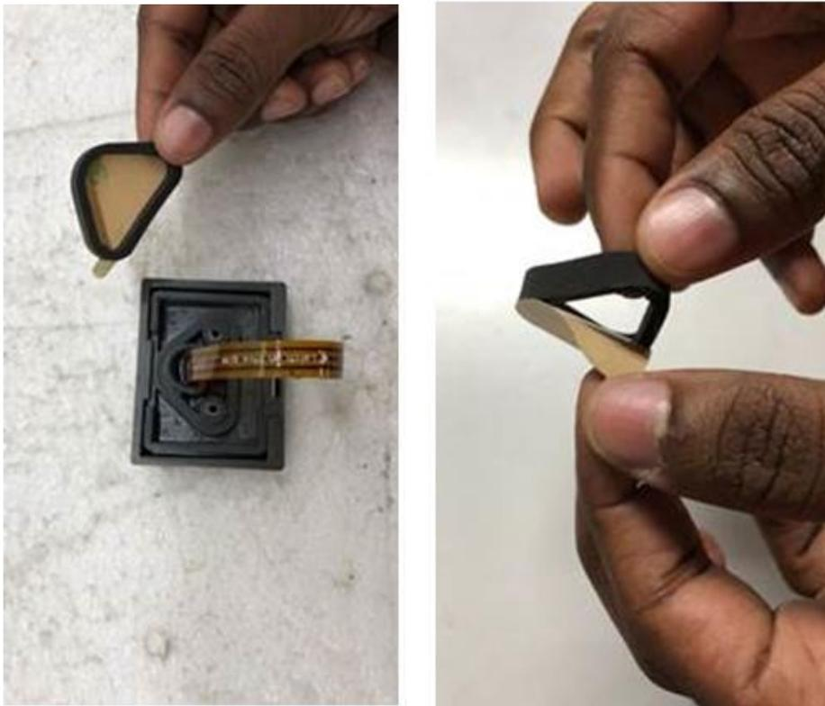
18. Apply and stick the adhesive side of MP1301 replacement gasket to each of the paddles.
