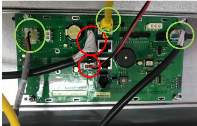
3. Remove and discard the below cables (circled) from the Wayne CPU board
