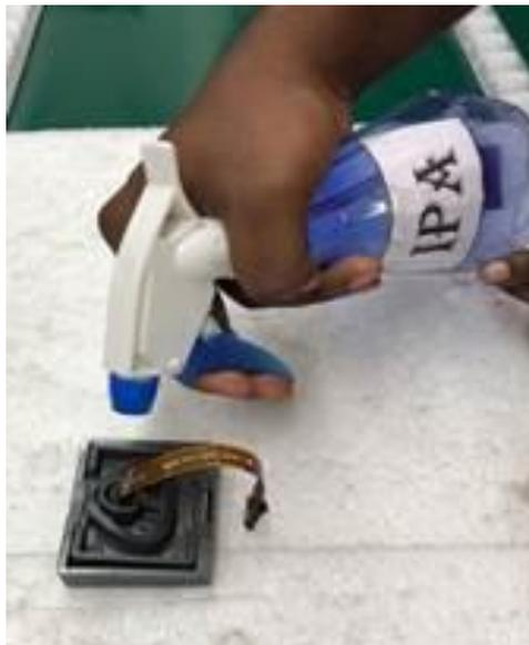
16. Peel off the existing gasket and clean the surface completely (ensure no residue remains), using a flat scraper if required. Take care not to damage the nearby parts, such as the ribbon
