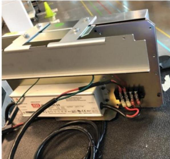
2. Install the Helix PSU Assembly with the Dispenser InvencoLink facing the installer on the B side of the dispenser (side opposite the pump controller board).
