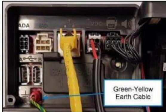
2. Use cable ties to tidy up the installation. Excessive lengths should be bundled and tied so they stay inside the pump cabinet frame.
