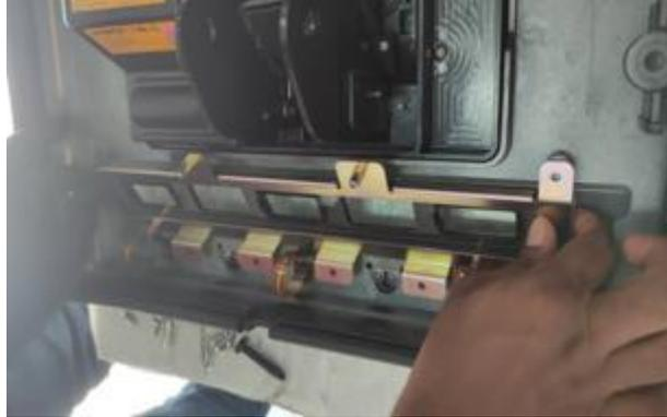
26. Screw the metal bracket with the glass cover in place with MS0176 (4pcs removed in earlier step 12 of this section and 4pcs from the kit). All eight screws are the same so can be used in any position.
