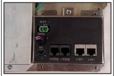
4. Take the four MS0143 Screws from the InvencoLink converter Retro-Fit Kit package and insert them into the four holes on the InvencoLink converter:
