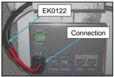
8. The installation of the InvencoLink converter is now complete. Discard the packaging for the InvencoLink converter and refer back to the installation instructions for the particular OPT Retro-Fit Kit with which you were working.
