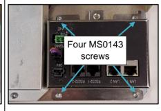
5. Tighten all four screws carefully to secure the terminal cover and InvencoLink converter in place. You may need to jiggle the parts a little to get a nice alignment.
