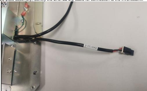
7. Insert the black connector on the EK0122 DC cable into the 1x3-way "24V" socket on the top of the InvencoLink converter.
