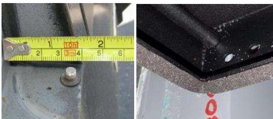
Fig 4.11 – Base of Retro-Fit Kit Door seated over lower hinge pin
