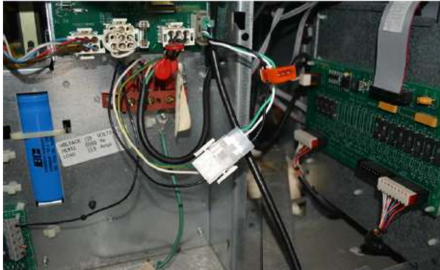
Fig 4.4g – main AC power line attached to the Y cable
