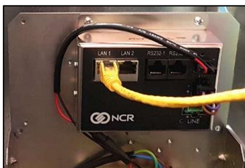
Fig 4.7– Connecting EK0131 to the InvencoLink Converter (Side-A)
