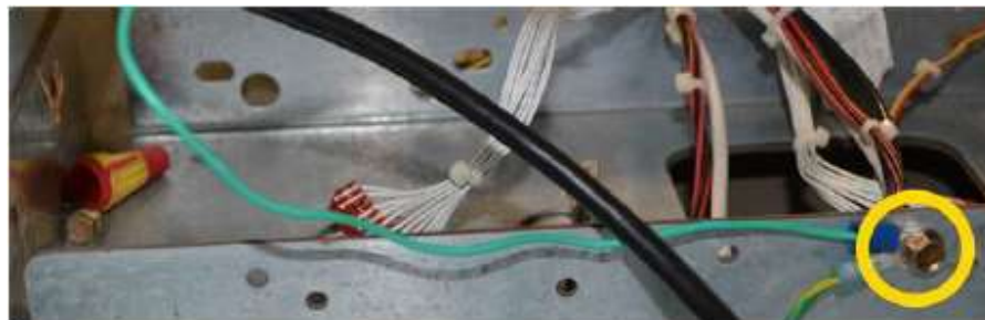
Fig 4.4d – Bolt with attached ground
