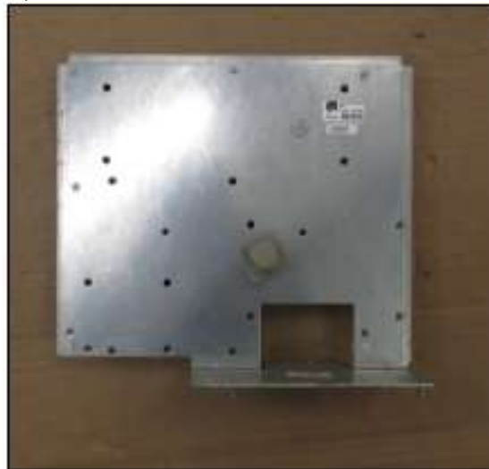
Fig 2.15e – CRIND Control Bracket after removal
