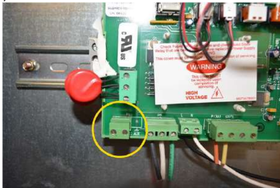
Fig 4.4b – P1 terminal on the Power Control Module
