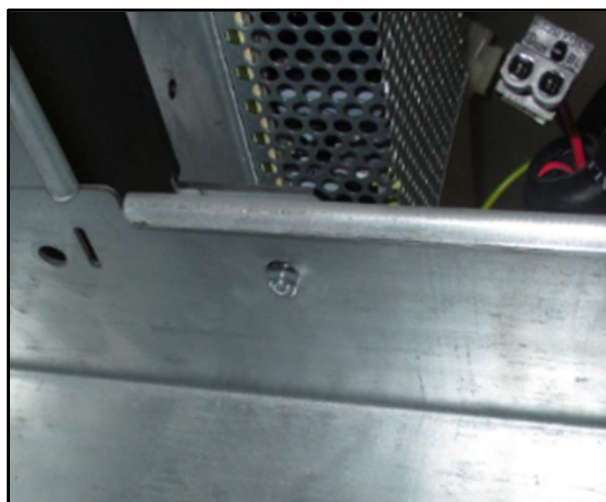
Fig 4.2 – Nuts for PSU Plate assembly (One side only shown)
