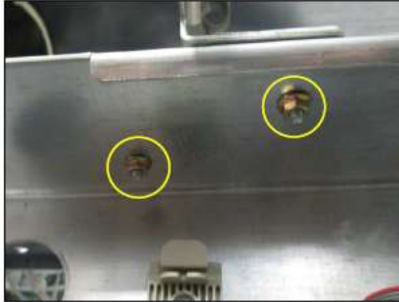
Fig 2.15d – Location of the CRIND Control Bracket nuts
