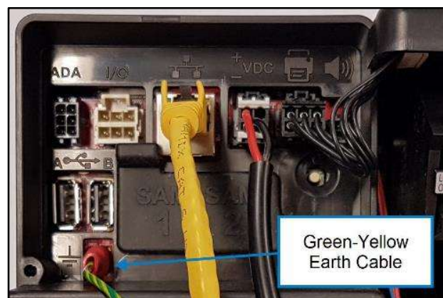
Fig 4.17– Connecting the earth cable to the OPT
