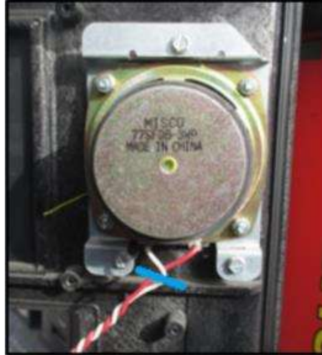
Fig 2.7 – Cut the speaker wiring
