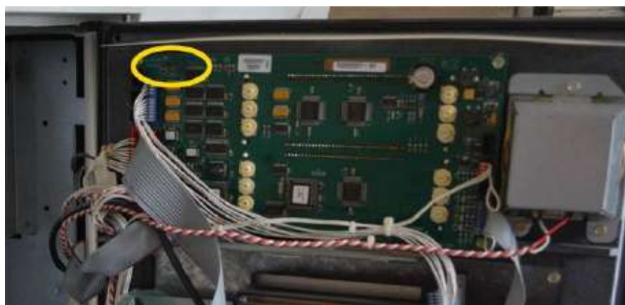
Fig 2.2d – Jumper present at JP5 (Side-B)
