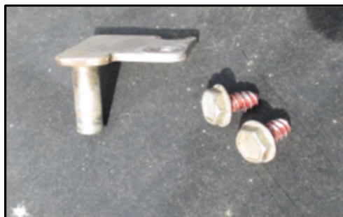
Fig 2.11 – Upper hinge pin and screws
