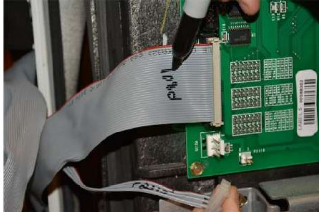
Fig 2.3a – Marking the cables
