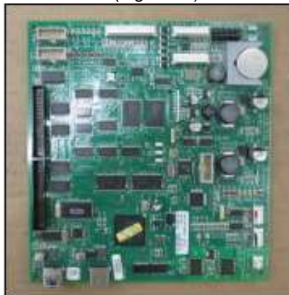
Fig 2.15c – CRIND Control Node after removal
