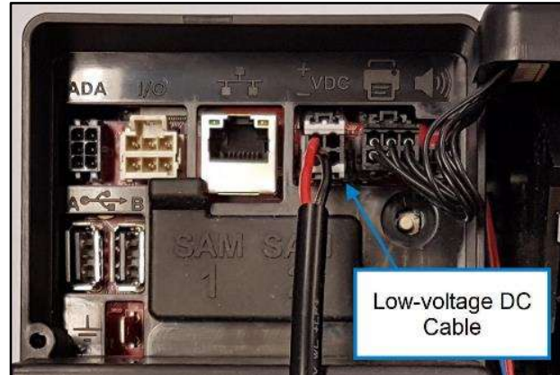
Fig 4.15– Connecting the DC cable
