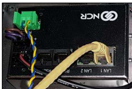
Fig 4.10– Connecting EK0140 to the InvencoLink Converter
