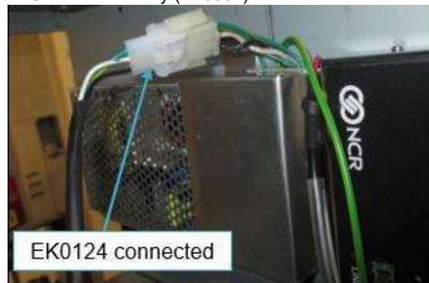
Fig 4.3b – Connecting EK0124 to the PSU mounted on Plate assembly
