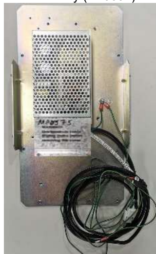
Power Supply Unit (PSU) mounted on Plate assembly (EZ0631):
