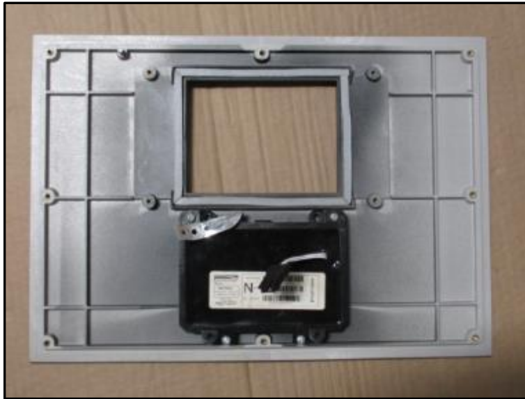
QVGA Panel and Customer keypad after removal
