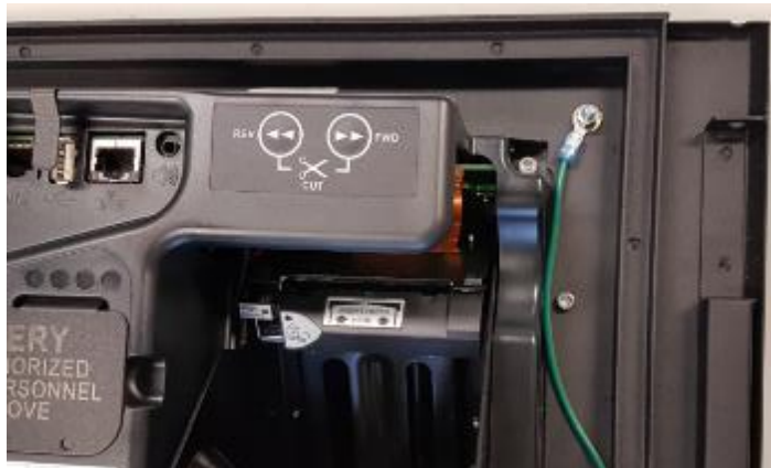
Fig. 2.2 – Connection secured with MN0029 #8-32 SEMS nut
