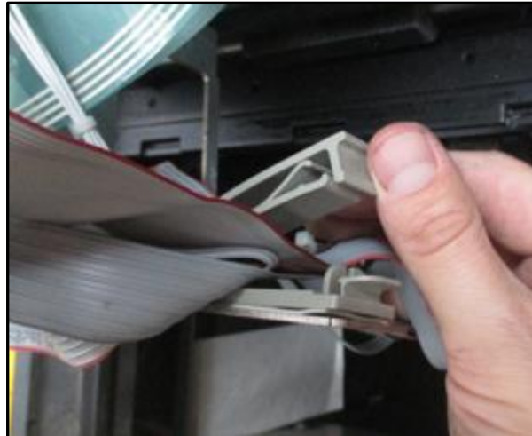
Fig. 1.3 – Unfasten cable restraints
