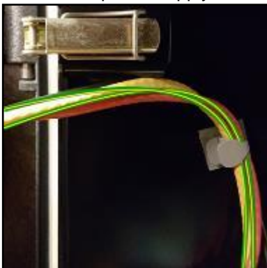
Fig. 3.12 – Cables retained in cavity near pump door clasp
