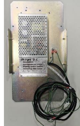
PSU plate mounting screws (MS0147) 6-32 x 5/16" machine screw SEMS – Quantity: 2
