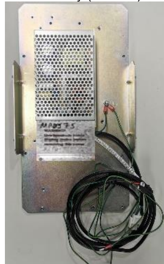
Power Supply Unit (PSU) mounted on Plate assembly (EZ0631):
