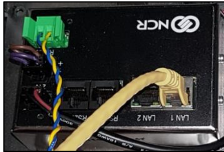
Fig 4.10– Connecting EK0140 to the InvencoLink Converter
