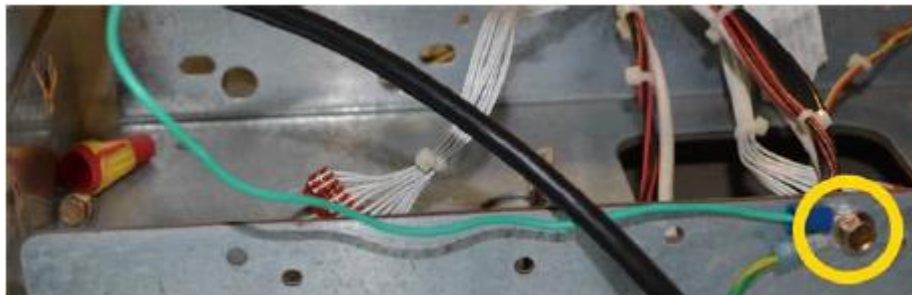
Fig 4.4d – Bolt with attached ground
