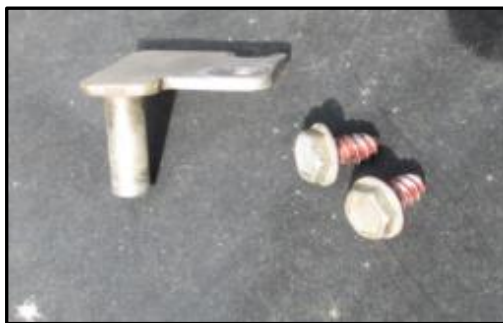
Fig 2.11 – Upper hinge pin and screws
