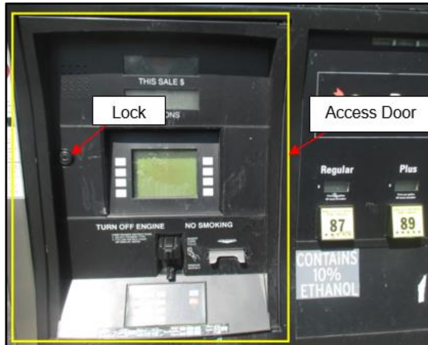
Fig 2.1 – Access door and lock location
