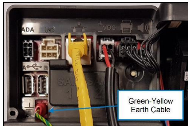
Fig 4.17– Connecting the earth cable to the OPT
