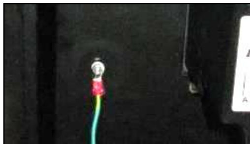
Fig 4.14– Installing ground wire onto RP00026-XX Retro-Fit Kit Door assembly
