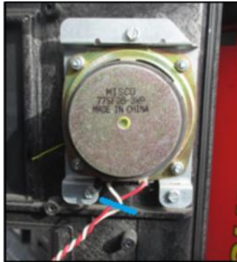
Fig 2.7 – Cut the speaker wiring
