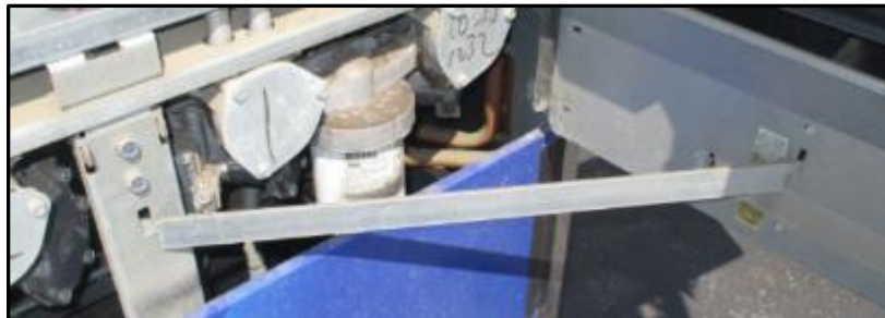
Fig 2.9b – Door prop inserted in prop position
