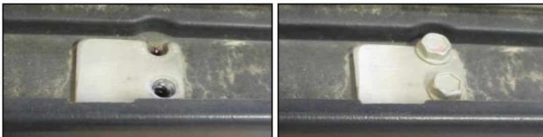
Fig 4.12 – Hinge pin installed, and screws inserted and tightened
