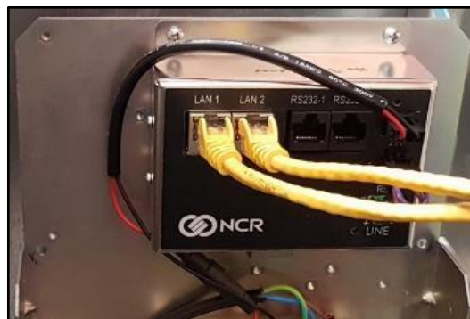
Fig 4.8– Connecting EK0131 to the InvencoLink Converter (Both Sides-A and -B)
