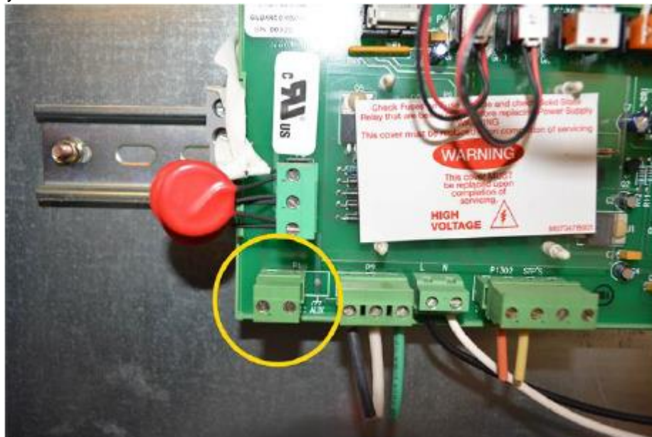
Fig 4.4b – P1 terminal on the Power Control Module
