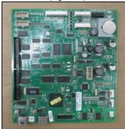
Fig 2.15c – CRIND Control Node after removal
