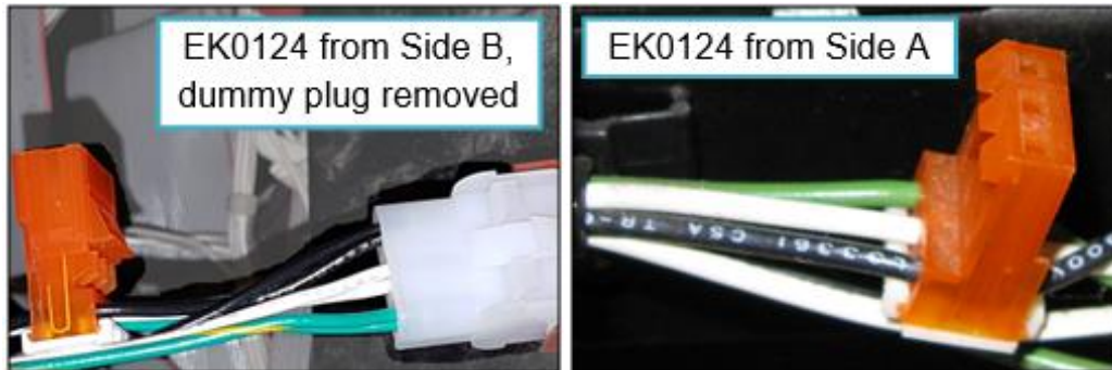
Fig 4.5 – Connections for EK0124's – Side-B
