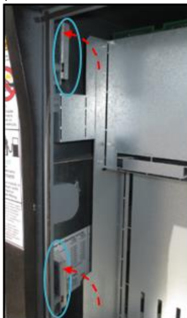
Fig 4.22 – Latching the dispenser's main door
