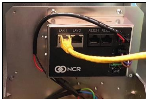
Fig 4.7– Connecting EK0131 to the InvencoLink Converter (Side-A)
