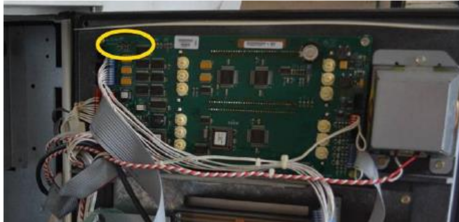
Fig 2.2d – Jumper present at JP5 (Side-B)
