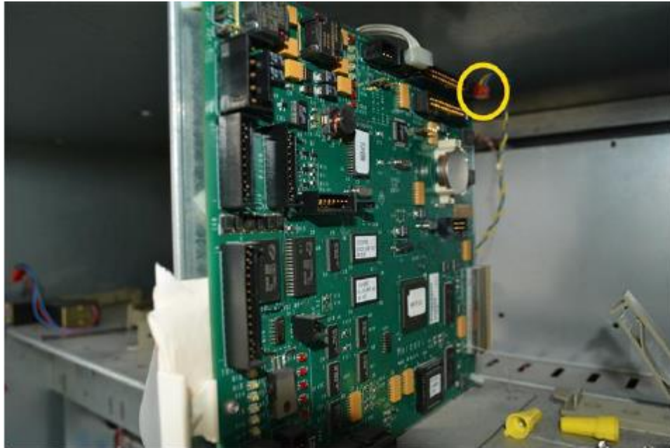
Fig 2.15b – Comm Two Wire from the CRIND control node board
