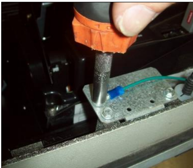
Fig. 6.10 – Attach grounding cable.
