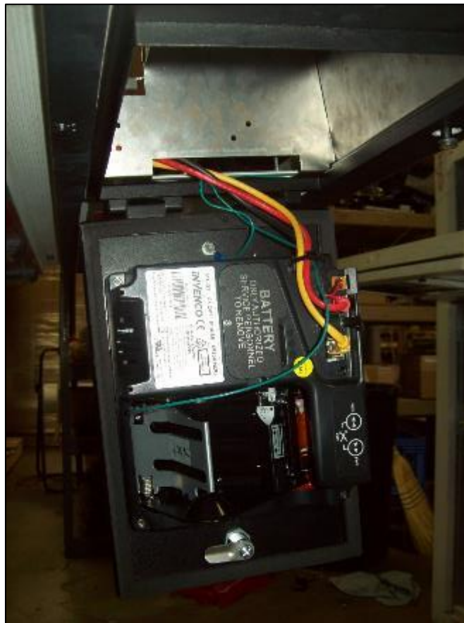
Fig. 6.18 Unlock the RFK and allow the OPT to hang freely.
