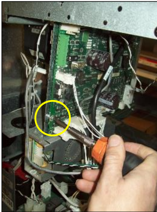
Fig 4.12.2e – Temporarily detach the Computer Board.
