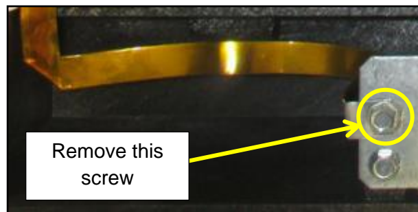
Fig. 4.9 – Location of the ground strap screw
