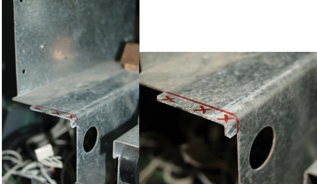
Fig 4.12.1d – Mark the area to cut away.
