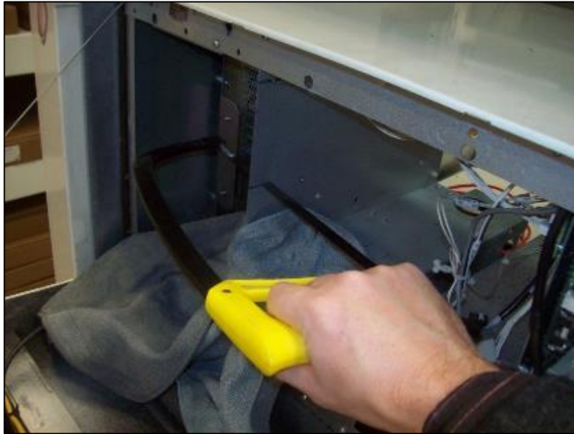
Fig 4.12.2i – Make two hacksaw cuts where indicated on the decal.
