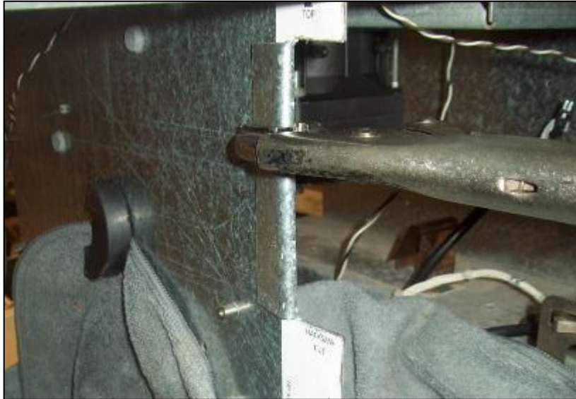
Fig 4.12.2k – Crimp bend flat using Standard Vice Grips.
