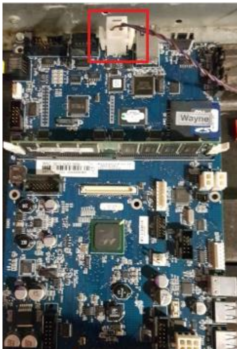
Fig. 4.11.1b – Location of the Q-CAT board
