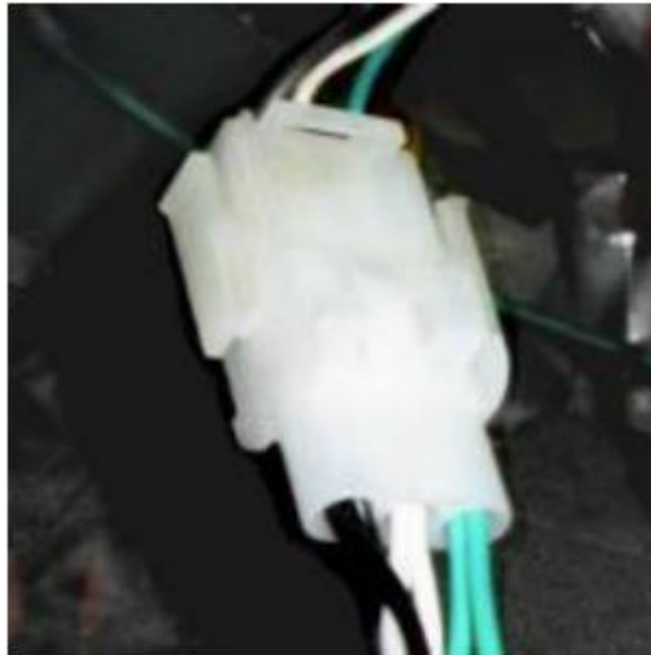
Fig. 6.26 – Connect the Plug removed in Step 22 to EK0137
