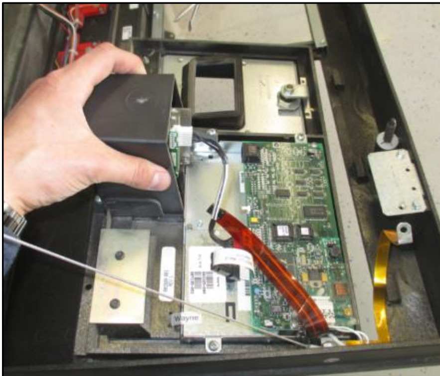
Fig. 4.10b – Grab the card reader and remove the assembly
