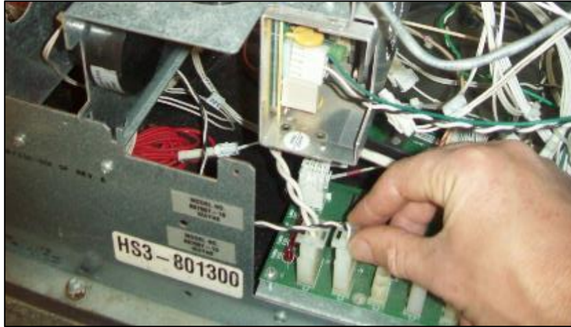
Fig 4.13.1e – Reconnect the Power Cable.
