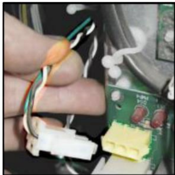
Fig. 6.22 – Unplug the mains connector from the relay board
