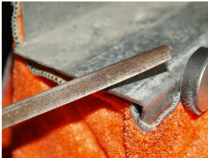
Fig 4.12.1g – File off sharp edges onto the drop cloths
