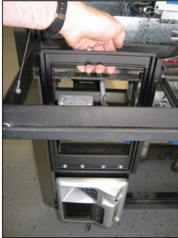
Fig. 6.4 – Bringing the frame through the opening
