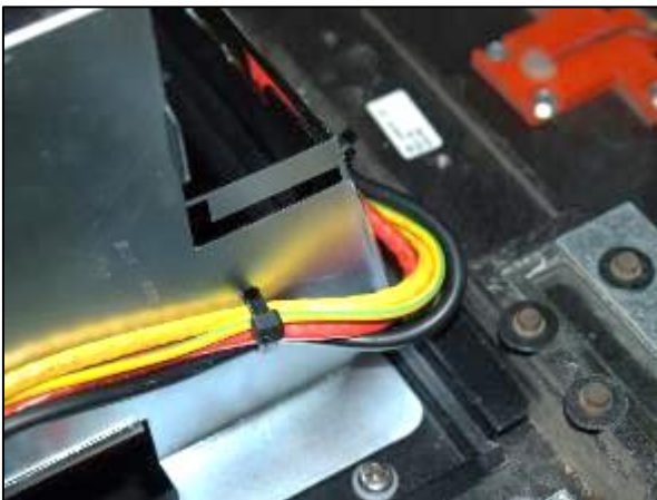
Fig. 6.20a – Keep cables clear of corner.
