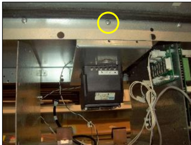
Fig 4.13.2d – Screw Location Side B.
