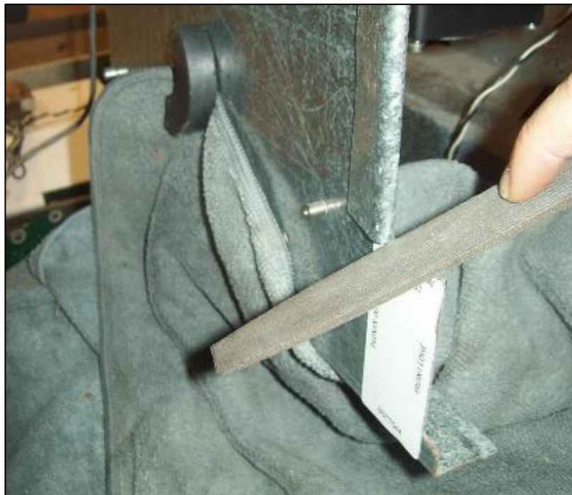
Fig 4.12.2l – File off sharp edges onto drop cloth.
