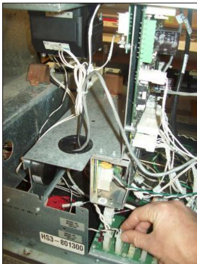
Fig 4.13.2e – Reconnect Power Cable.
