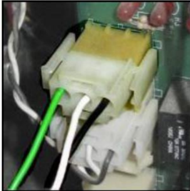
Fig. 6.25 –Plug the double connector end of the EK0137 to the relay board
