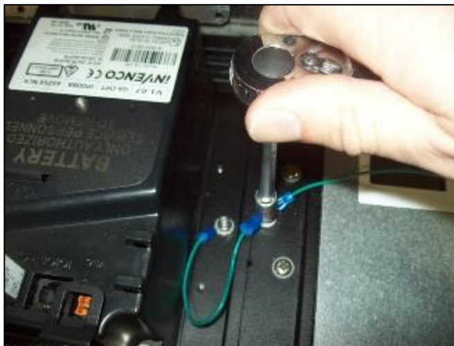
Fig. 6.11 – Temporarily detach grounding nut.
