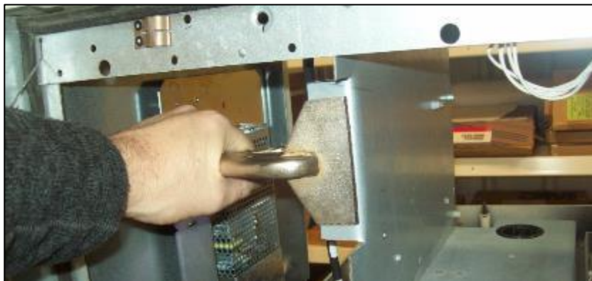
Fig 4.12.2j – Initial bend using 3" Wide Jaw Vice Grips.
