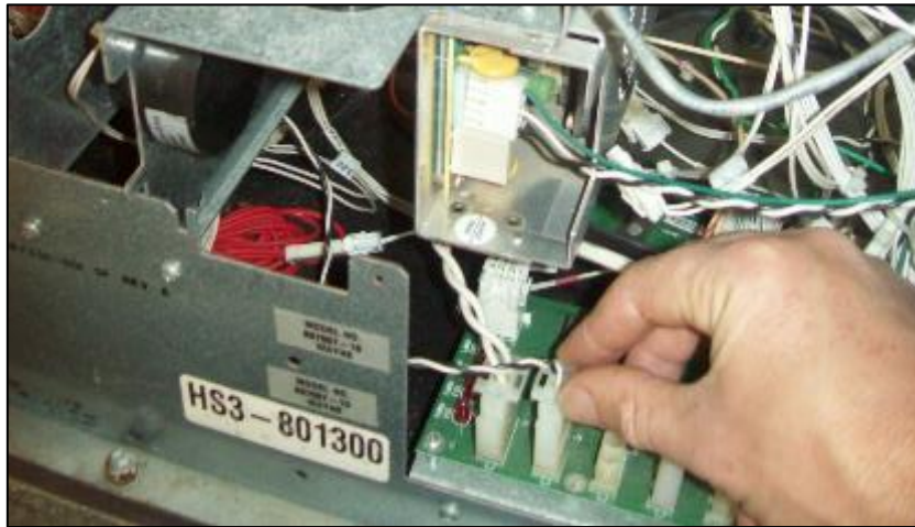
Fig 4.13a – Disconnect power cable.
