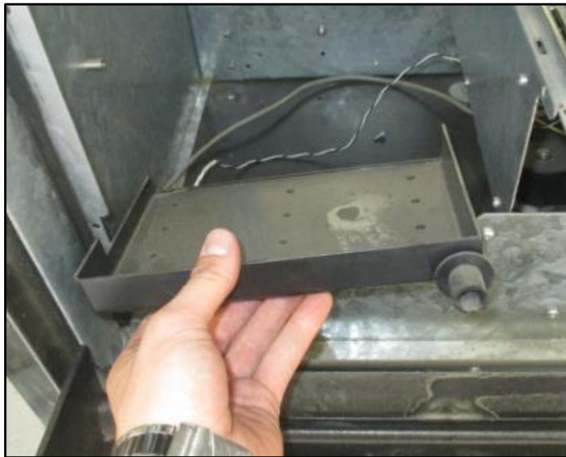
Fig. 4.14b – Removal of water catch tray
