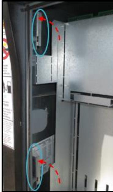
**Fig 4.22 – Latching the dispenser's main door**
