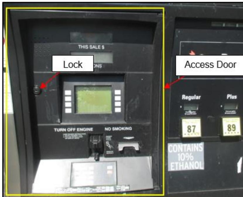
Fig 2.1 – Access door and lock location
