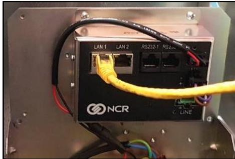
Fig 4.7– Connecting EK0131 to the InvencoLink Converter (Side-A)
