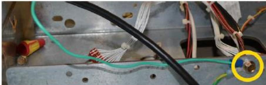
**Fig 4.4d – Bolt with attached ground**
