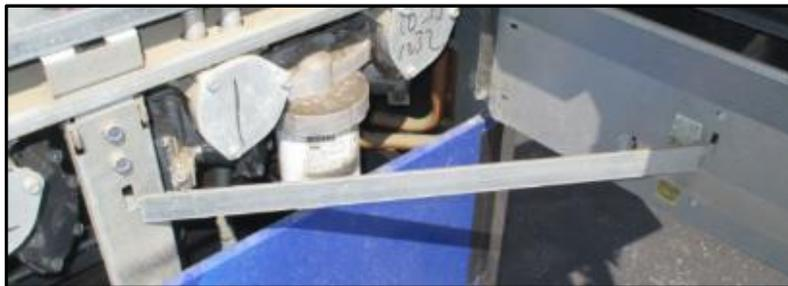
Fig 2.9b – Door prop inserted in prop position
