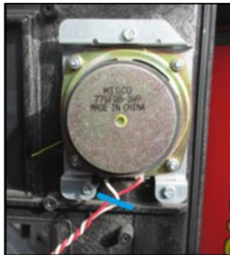
**Fig 2.7a – Cut the speaker wiring**
