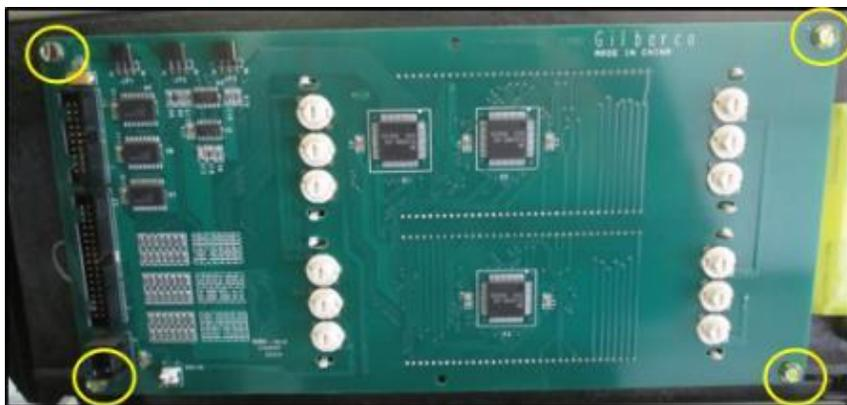
Fig 2.4 – 1/4" hex head screws on main display
