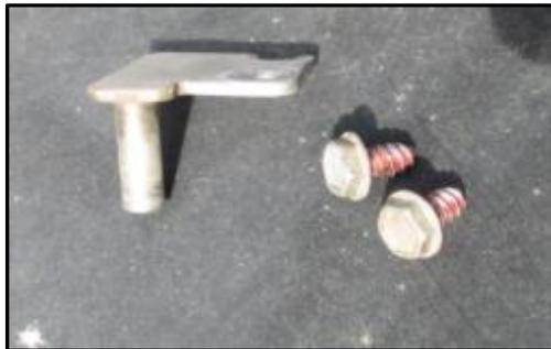
**Fig 2.11 – Upper hinge pin and screws**
