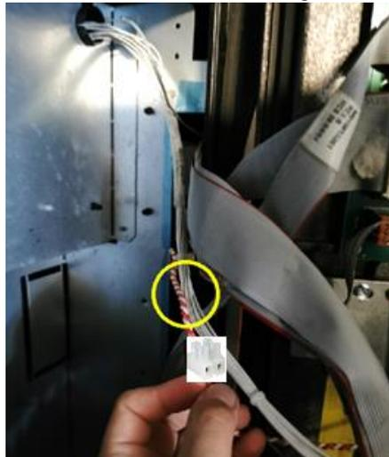
**Fig 2.7c – Cable (zip) tie and terminal block location**
