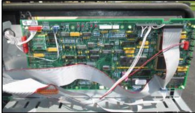
**Fig 2.12 – Logic board with cabling plugged in**
