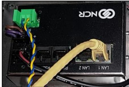
**Fig 4.10– Connecting EK0140 to the InvencoLink Converter**
