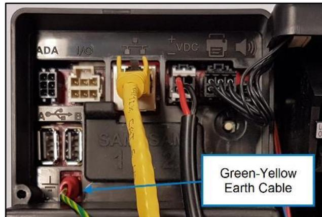
**Fig 4.17– Connecting the earth cable to the OPT**
