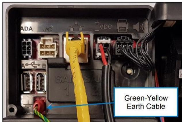
**Fig. 3.7 – Plug-in Earth Cable**
