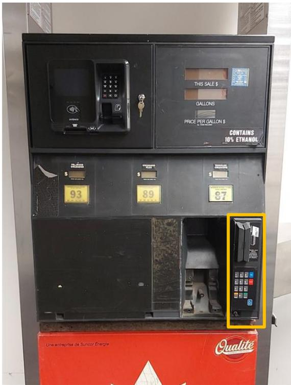
4. Using a 3/16" Hex key, undo the retaining bolts located along the bottom edge of the main door. Depending on the model and dispenser setup, there could be between two to four bolts to remove. The bolts should be captive but may fall out. Do not discard these bolts. (Fig. 1.1)
