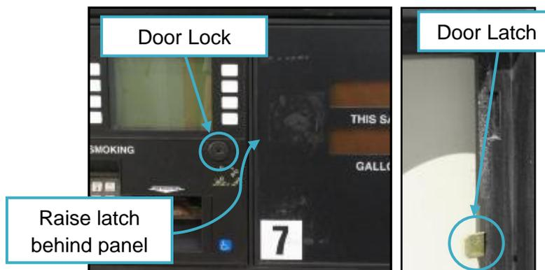
Fig. 1.2b – Unlock both option doors (Narrow)
