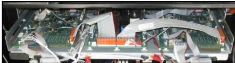
**Fig. 1.13c – CRIND boards on frame in pump**
