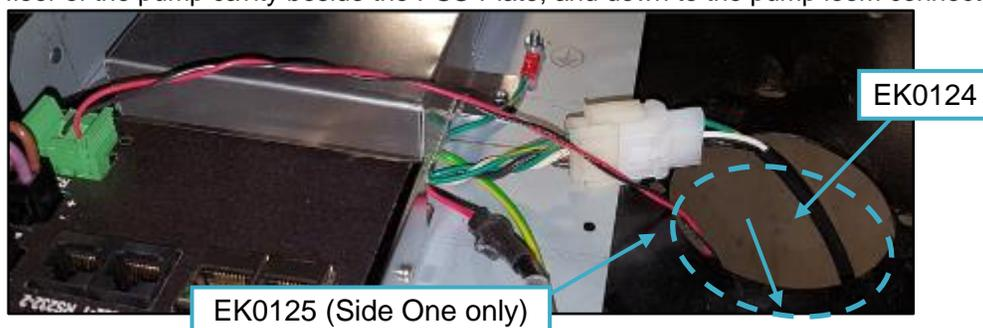
**Fig. 3.15 – Routing EK0124 (& EK0125 For Side One)**
