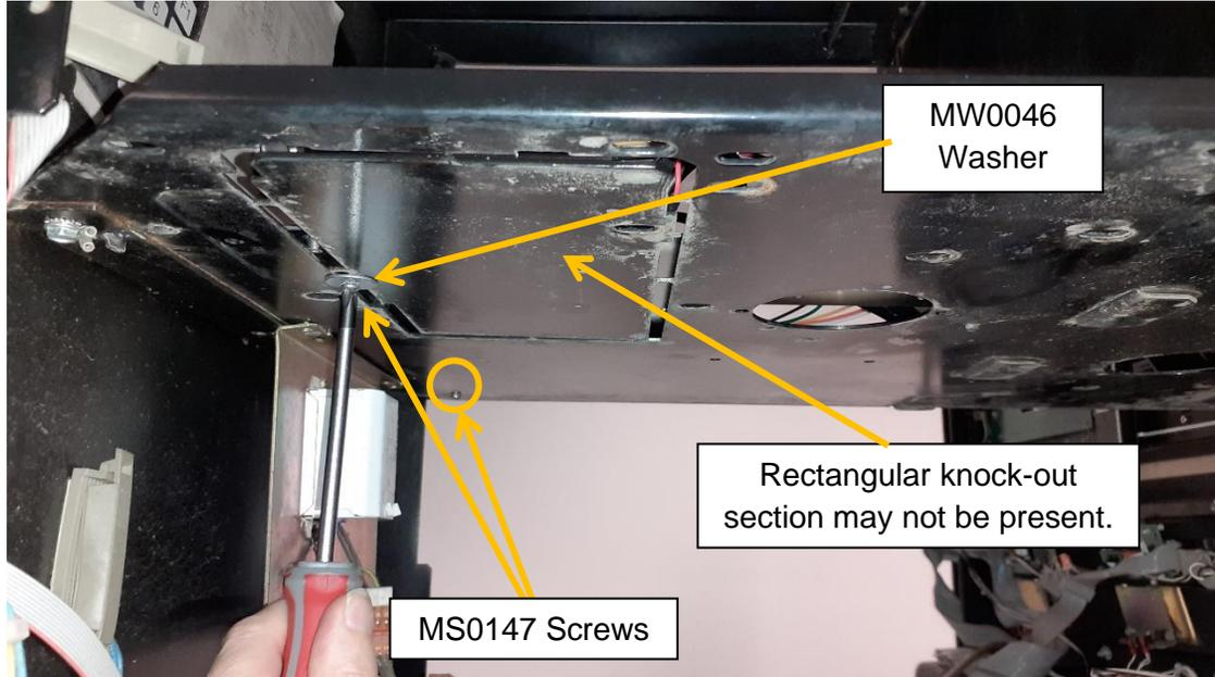
Fig. 3.2 – Plate secured with screws and a washer
