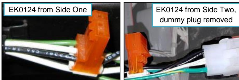
**Fig. 3.17 – EK0124 orange connectors to be joined together.**
