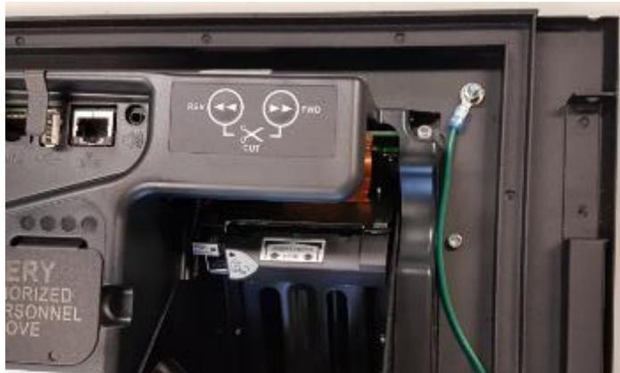
**Retrofit G6-300+InvencoLink GVR Advantage (US) Installation Guide****Fig. 2.2 – Connection secured with MN0029 #8-32 SEMS nut****4.2.2 Replace the Gasket on the Pump Door**
