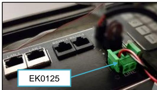
**Fig. 3.14 – Plug EK0125 into InvencoLink converter**
