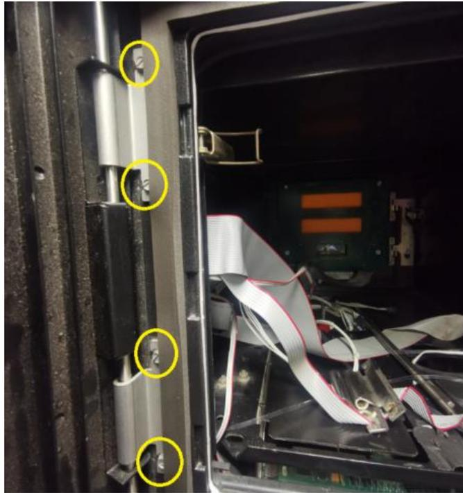
**Retrofit G6-300+InvencoLink GVR Advantage (US) Installation Guide****11.** Fit the replacement hinges (MP1080).
