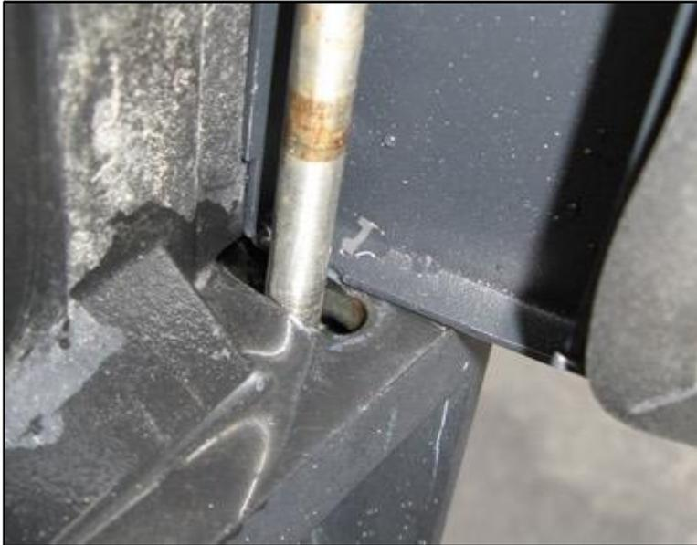
**Fig. 3.4 – Installing Hinge pin**
