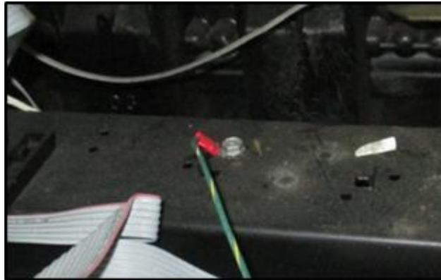
Fig. 1.13d – Unscrew ground wire
