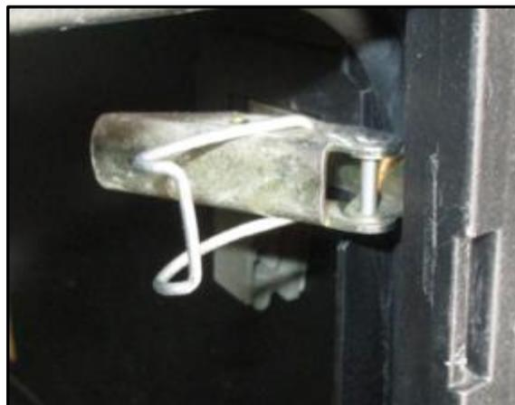
Fig. 1.10b – Door latch in the unlock position
