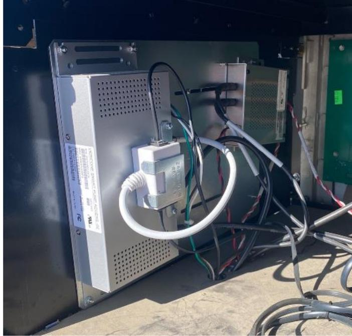
The current loop convert may be mounted separately on the side wall on its own by a single Philips screw:
