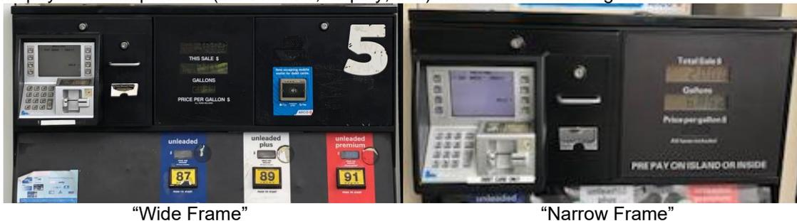
If the ADA V2 Box G6-300 (RF00101-XX) is being installed, also identify if the ADA Auxiliary Card Reader/ Keypad Module have been retrofitted. It will look like the following:
