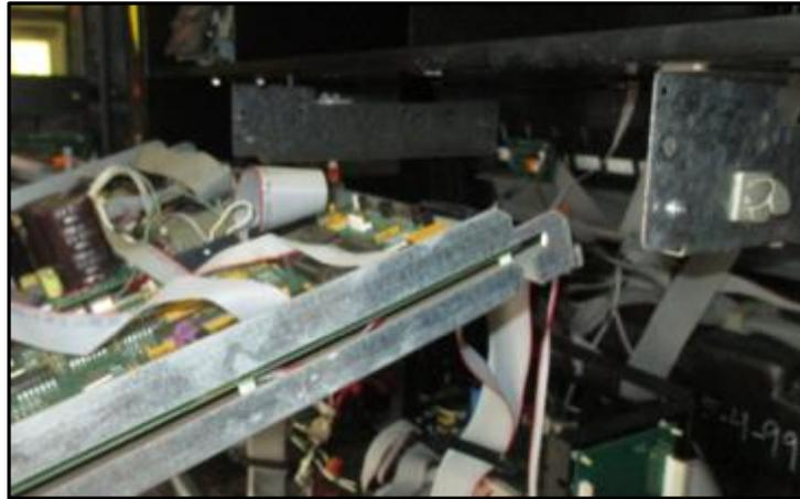
**Fig. 1.18b – Lift CRIND rack up and pull out**
