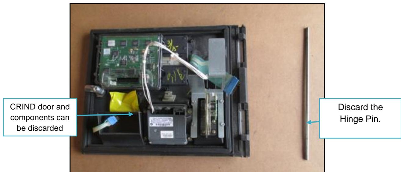
Fig. 1.12c – CRIND Door and hinge pin
