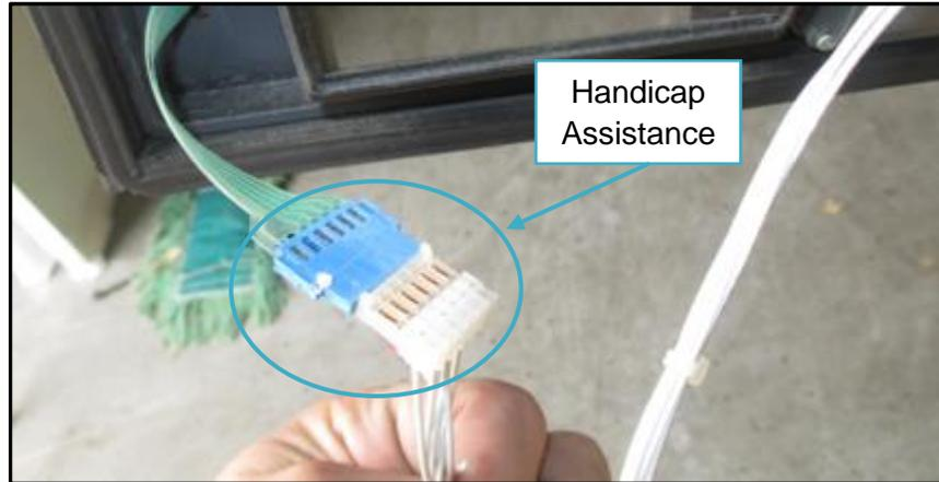
**Fig. 1.5- Unplug handicap assistance cable**
