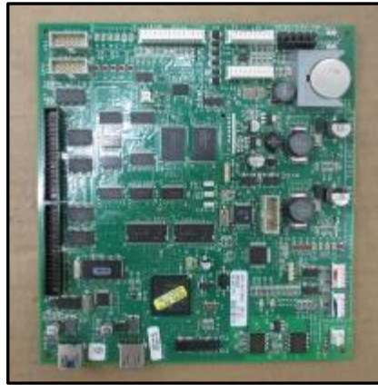
Fig 1.19 – CRIND Control Node after removal
