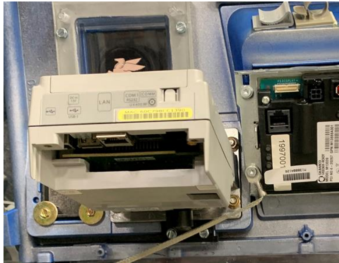
Fig 1.9b – Encore 700S Location of Card Reader plate screws
