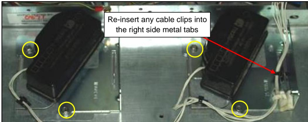
**Note:** For any of the holes that have not been used before (i.e. there is no thread in the hole), re-use one of the original screws instead. Check this before attempting to force a supplied screw into the hole. The supplied screws will not work to cut a new thread.
