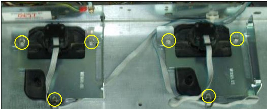
3. Using a 5/16" socket or nut driver, install and tighten all six MS0166 screws (circled above) to secure the Foot Brackets to the cabinet. Take care not to pinch any cables.
