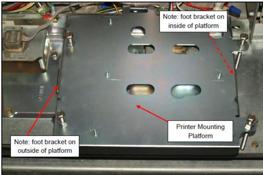
**Note: Ensure the Rear Tab on the rear of the Printer Mounting Platform is on the inside of the Cabinet Rail:**
