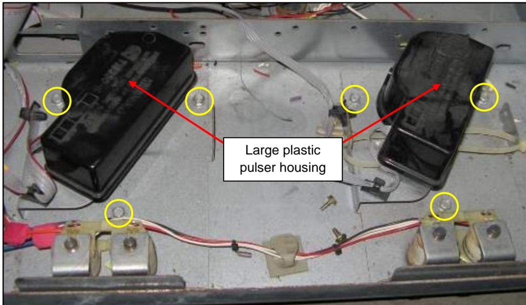
If the pulsers have large plastic bodies on top of a large metal base that extends to the front of the dispenser and is fitted with 3 screws, proceed to Step 6.2.5.
