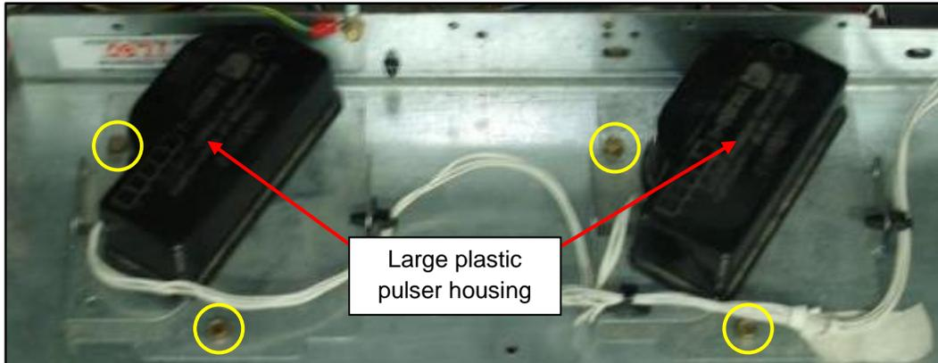
If the pulsers have large plastic bodies on top of a metal base with 2 screws (circled above), proceed to Step 6.2.4
