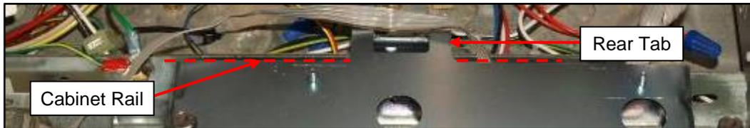
2. Place an MW0046 #10 Washer onto an MS0166 #10-32 x 3/4" Hex Head Screw, and insert the screw through the slotted hole in the cabinet rail and into the Cage Nut on the rear tab of the Printer Mounting Bracket. If the nut is not visible through the slotted hole in the cabinet rail, slide the Cage Nut up or down until it can be seen. To fit the screw, use a 5/16" nut driver or socket with a shaft of at least 10". Do not tighten the screw.
