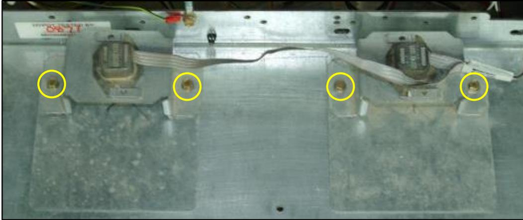
c. Lift the pulser off the shaft. Retain the pulser:
