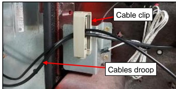
16. Use cable ties to secure any loose cables.
