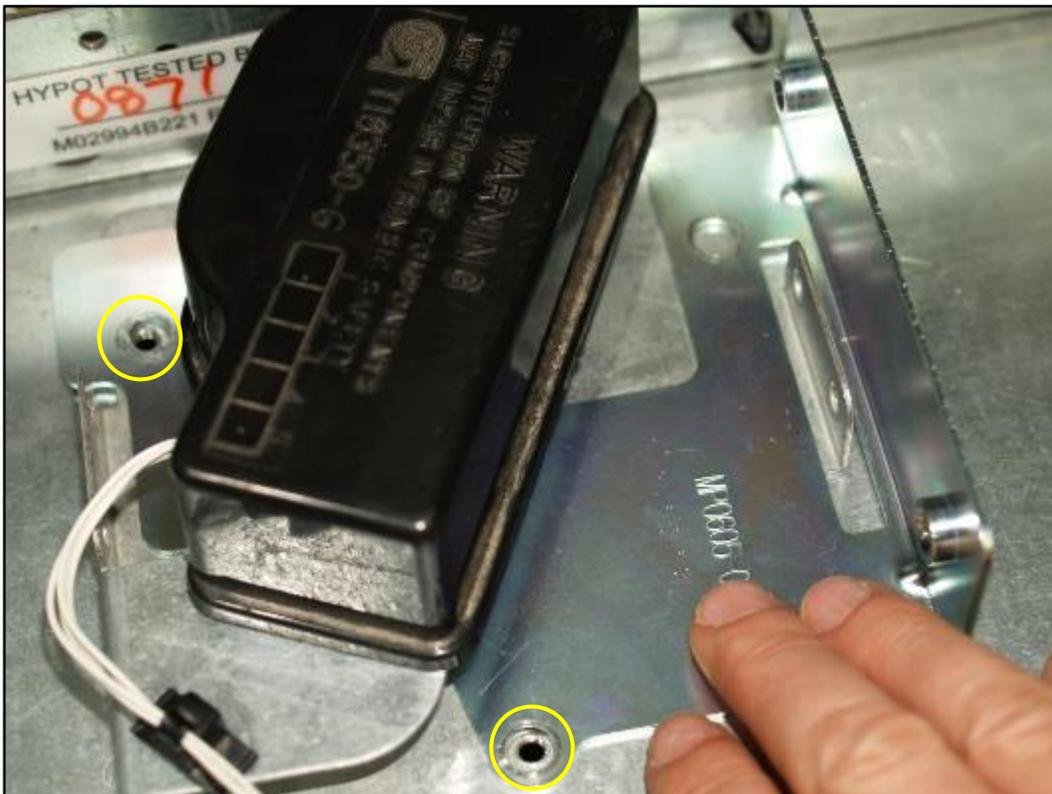
c. Using a 5/16" socket or nut driver, install and tighten all four MS0166 screws (circled above) to secure the Foot Brackets to the cabinet. Take care not to pinch any cables.
