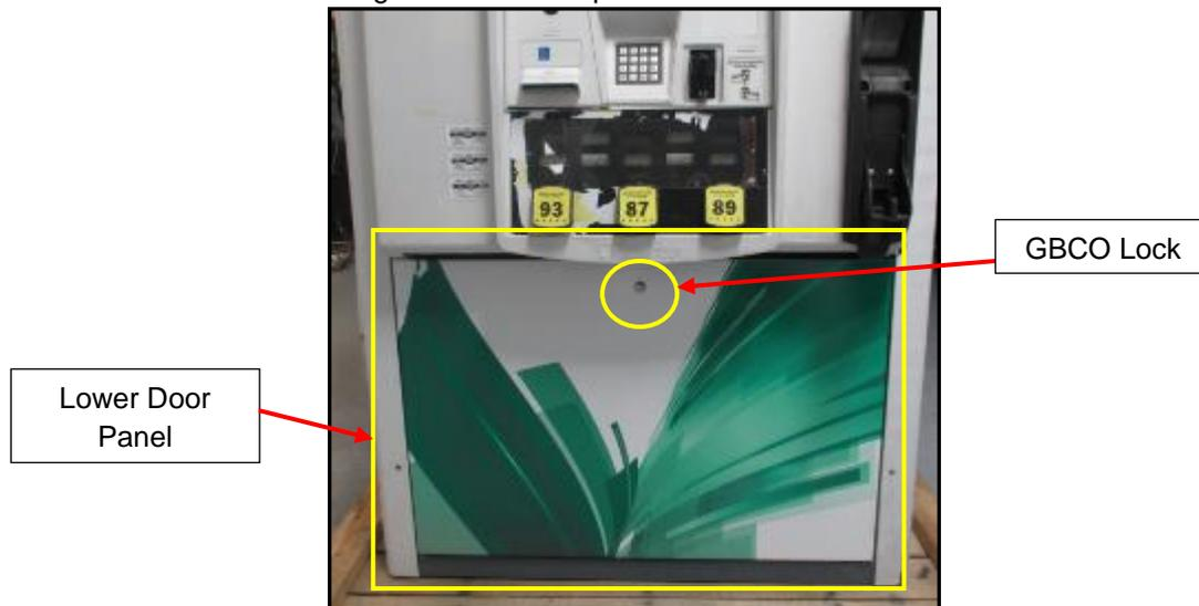
2. Undo the lower door latch located underneath the left-hand side of the Main Dispenser Door.
