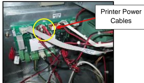
15. Remove the Printer Cables from the Dispenser. Unfasten any cable restraints necessary and re-fasten them after the printer cables are removed.
