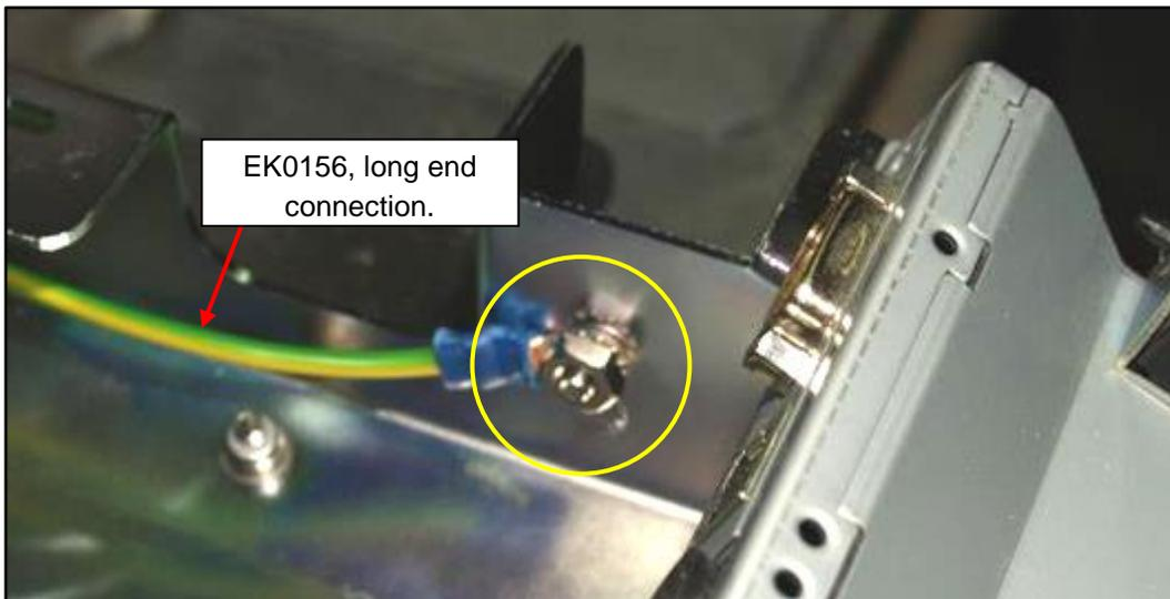
5. Pass the rest of EK0156 through the void behind the Printer Assembly into the pump cabinet.
