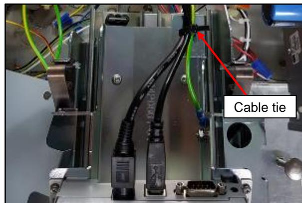
11. With the printer mechanism all the way out, cable-tie the three cables (EK0157, EK0117, EK0156) onto the pump's equipment shelf in the location shown. Also clip the EK0156 earth cable into the cable clip to the left of the cable tie:
