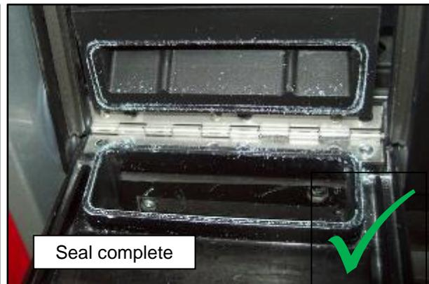
**Note:** A dual chalk ring should be visible on all four sides around the printer gasket opening.
