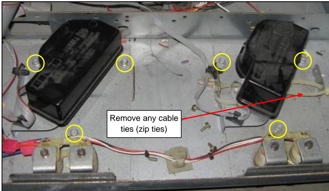
3. Use Needle Nose Pliers to disconnect any plastic cable clips from the right side metal tabs. Retain these clips to be re-installed later.
