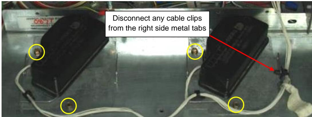
3. Use Needle Nose Pliers to disconnect any plastic cable clips from the right side metal tabs. Retain these clips to be re-installed later.
