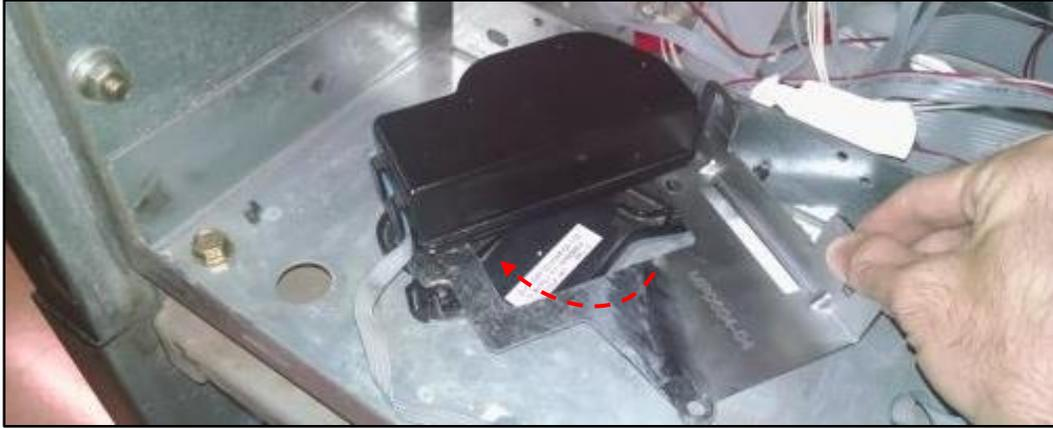
**Note:** Verify the correct foot bracket is installed to the correct side. The install steps are the same but the slot configuration of the foot bracket are different from left to right side.
