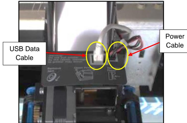
7. Unfasten the cable restraints on the Printer Assembly. There is one on the top of the Printer Shield, one on the side of the Printer Mechanism, and one on the back-side of the Printer Mechanism.
