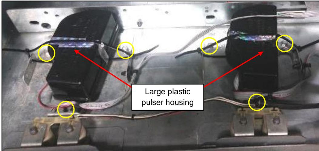
If the pulsers have large plastic bodies on top of small metal bases fitted with 3 screws (circled above), proceed to Step 6.2.6
