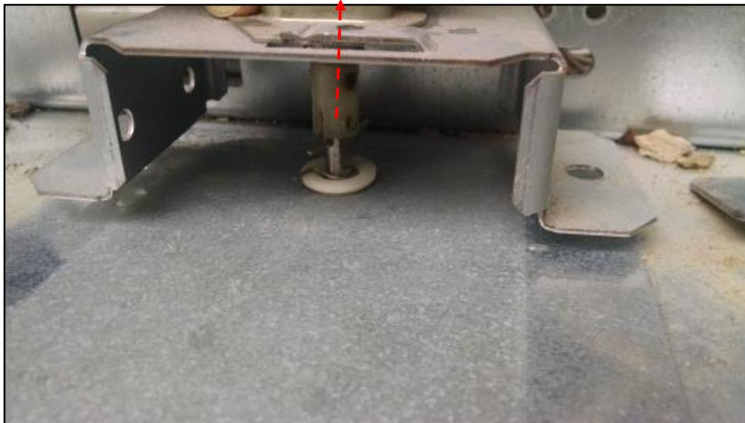
d. Un-latch the pin on each pulser by swinging the pin up and sliding it out. Retain the two pins.
