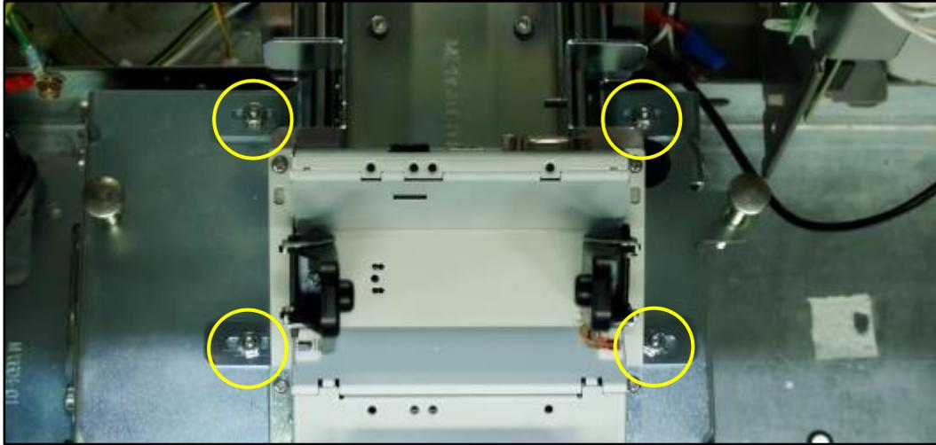
2. Check clearance between the Printer Assembly and the Printer Door.
