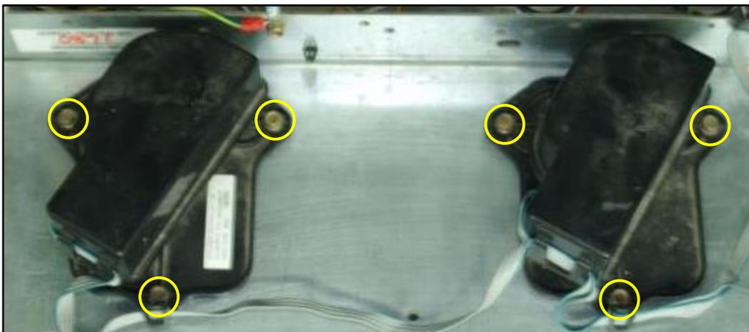
1. Using a 5/16" socket or nut driver, remove all screws holding the pulser (circled above). Retain the pulser and the screws.
