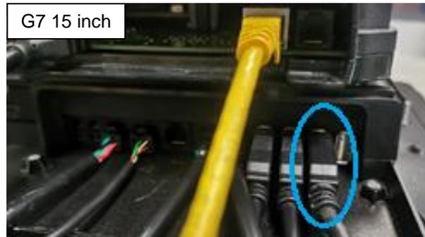
14. Plug EK0117 into the “PRINTER PWR” socket on the G7 or the G7 15 inch SDC:
