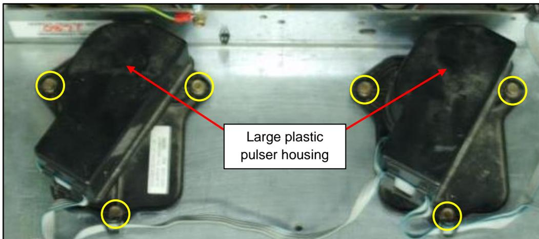
If the pulsers have a large plastic housing on top of a plastic base with 3 screws (circled above), proceed to Step 6.2.3
