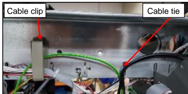
12. Pass the EK0157 & EK0117 cables to the right, under the equipment shelf and above other modules, using the existing cable clips for support:
