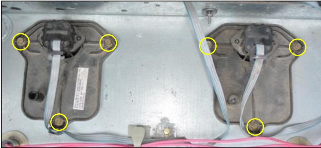
**Note:** Verify the correct foot bracket is installed to the correct side. The install steps are the same but the slot configuration of the foot bracket are different from left to right side.
