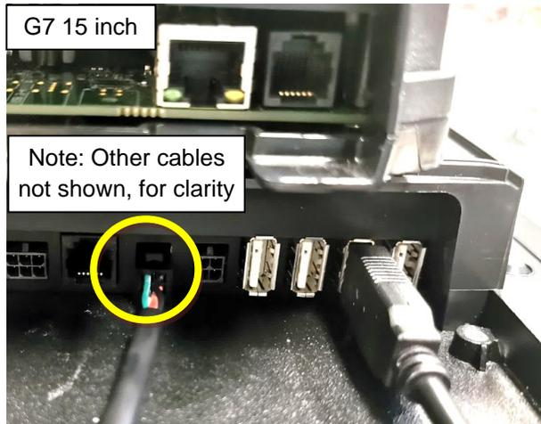
15. Draw the cables gently away from the G7 or the G7 15 inch SDC, and secure them with the cable clip on the pump door, leaving the any excess as a droop where the cables cross the pump door hinge area:
