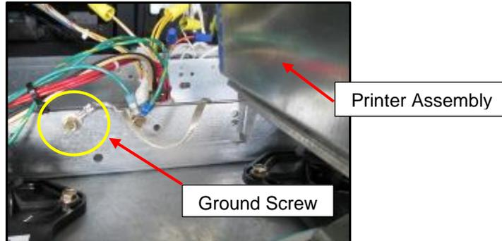
11. Slide the printer assembly back, so that it does not tip over when the mounting screws are removed in the next step.
