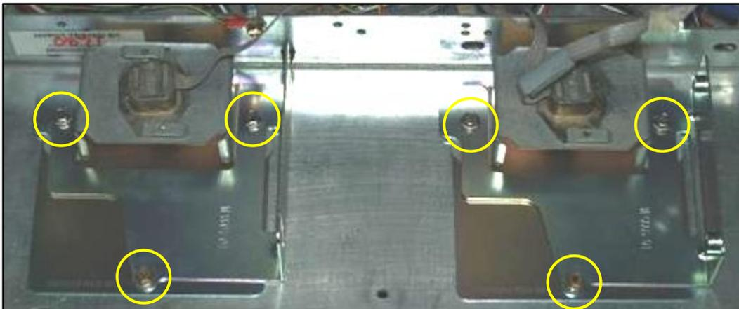
**Note: For any of the holes that have not been used before (i.e. there is no thread in the hole), re-use one of the original screws instead. Check this before attempting to force a supplied screw into the hole. The supplied screws will not work to cut a new thread.**
