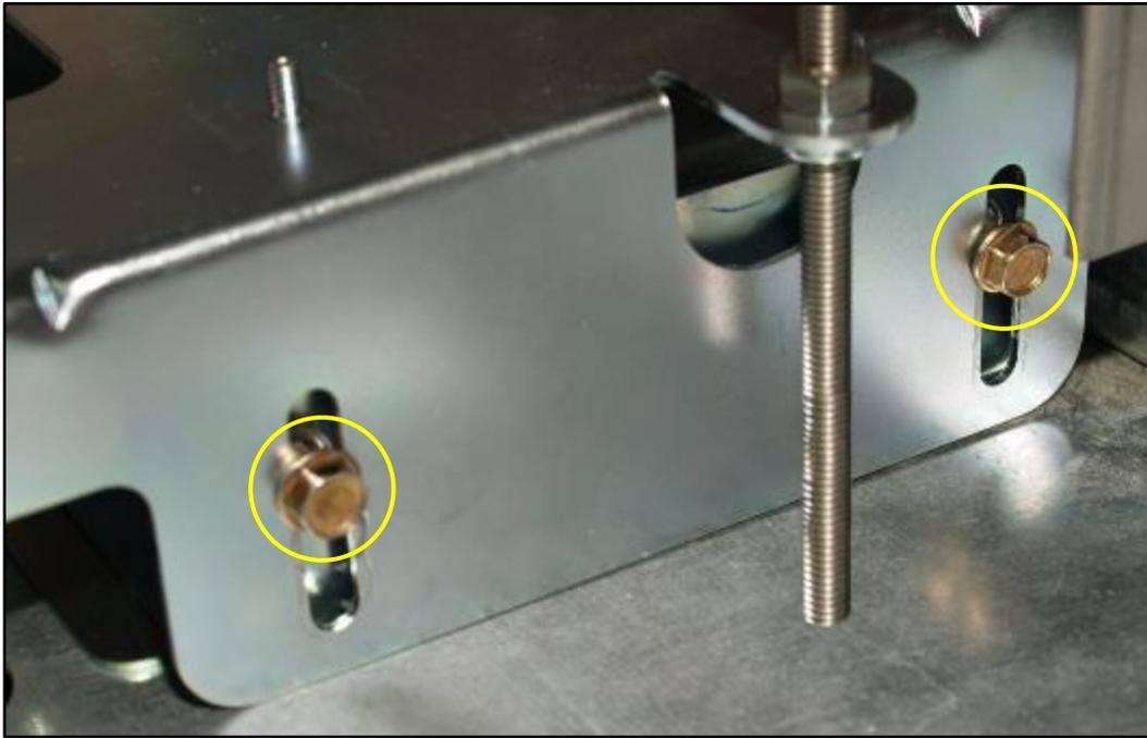
4. Insert two MS0177 M6x12 Sems Screws (circled below) in the left-hand side of the Printer Mounting Bracket, threading them into MP0604. Do not tighten the screws.
