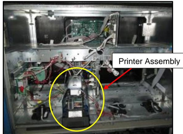
5. Pull the Printer Mechanism fully forward.
