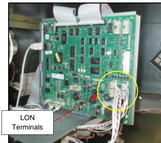
Fig 1.18a,b – LON Terminals, CRIND Control Node (left) & CPU Board (right)
