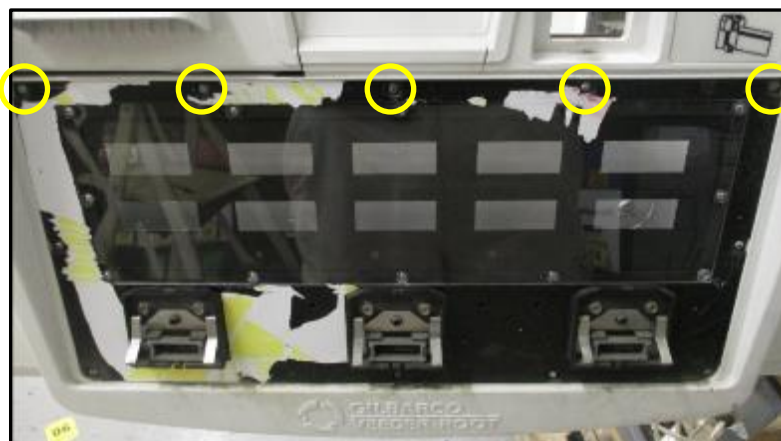
Fig 1.13 – Location of fastening screws on Product ID Plexi-Bezel
