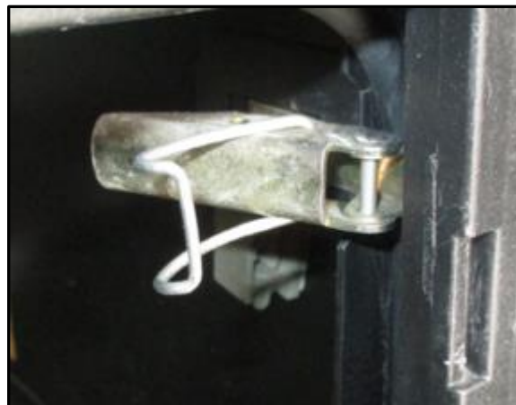
Door latch in the unlock position
