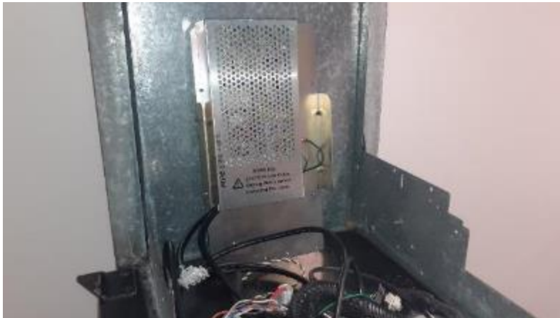
Place PSU Assembly EZ0703 inside pump.
