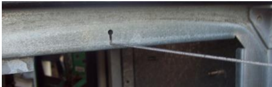
ABOVE: Tension cable door stay on a Vista 3V dispenser.
