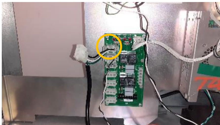
Connecting the Power Adapter Cable (EK0137) to Relay Board
