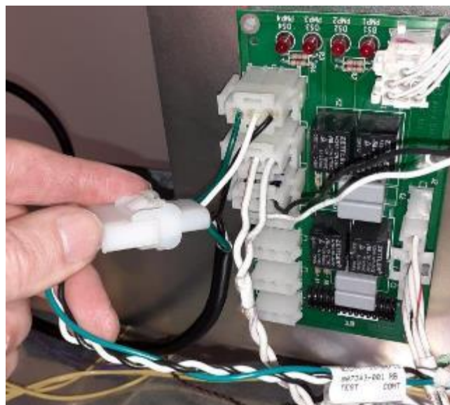
Reconnecting Power Supply to Relay Board in a daisy chain.
