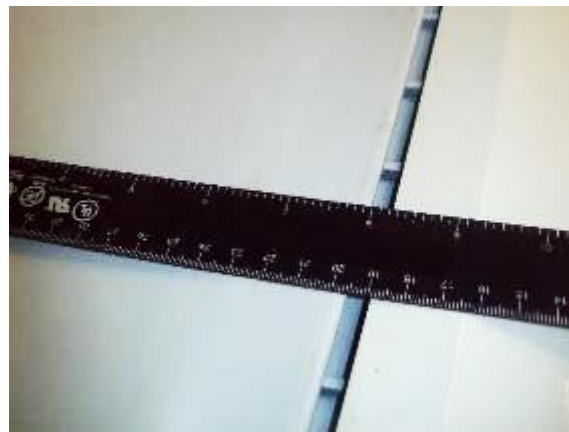
The 4V door gap at the top of the dispenser is around \frac{1}{4} " (6mm).
