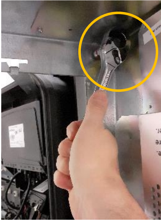
Re-tighten Top Hinge Bracket Nuts
