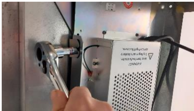
Tighten Nuts (MN0029) on both sides
