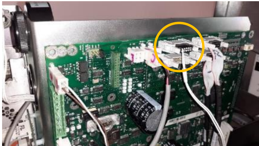
Reconnect Totalizer Cables to CPU board.
