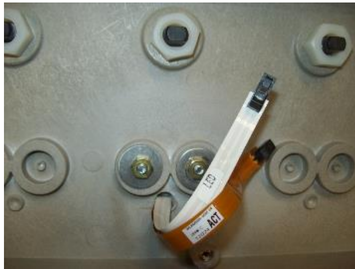
Fuel Grade Selector Button with two ribbon cables. The LED Plugs above the button are not removed with this type of Selector, as it has built in LEDs.
