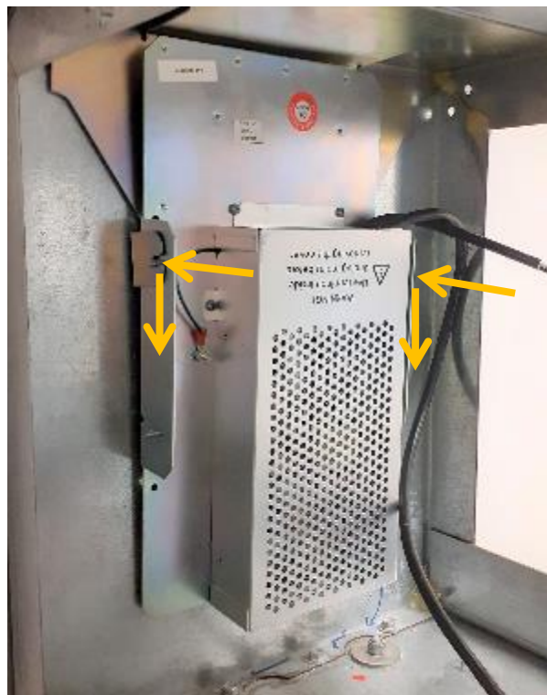
Hang PSU from Mounting Bracket
