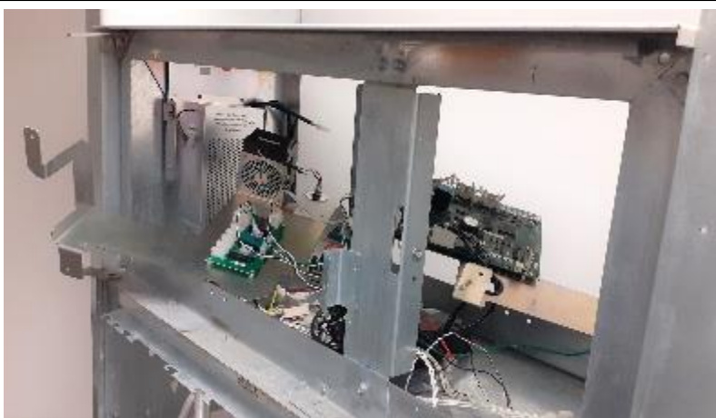
Place the Electronic Panel inside the pump
