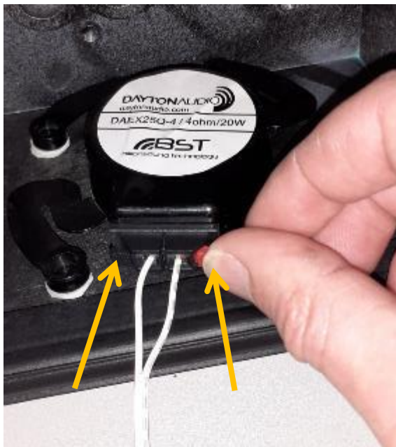
Press side levers to open cable clamps.
