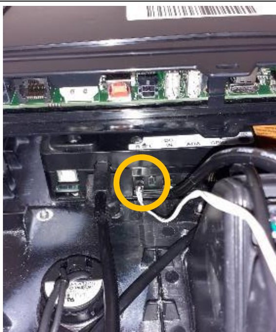
Press side levers to open cable clamps.
