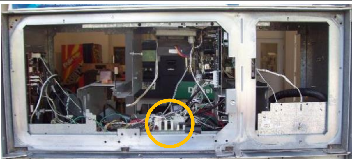
Relay Board location, Side A on a Vista 3V Wide Frame.
