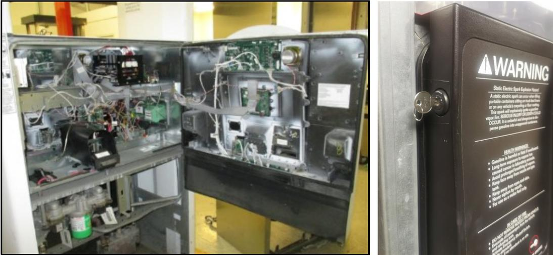
2. Do up the lower door latch located underneath the left-hand side of the Main Dispenser Door.
