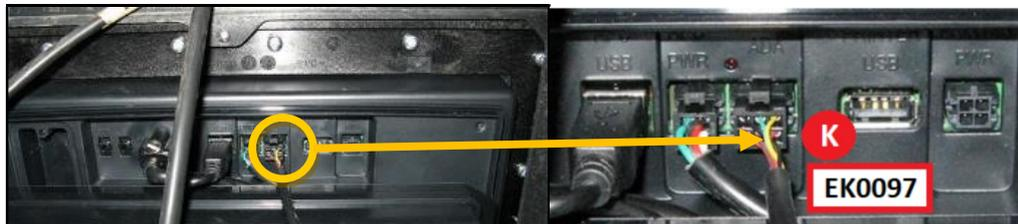
3. Detach the APC module that is mounted on the SDC module by undoing the four screws holding the APC in place (use a Philips #2 screwdriver). Retain these screws for re-use later during the installation steps. Cut any cable ties that are securing the cables connecting to the APC module as required. Temporarily hold the APC in one hand, while removing the cables connected to the SDC with the other (do not remove the cables from the APC), referring to the image in step 2:
