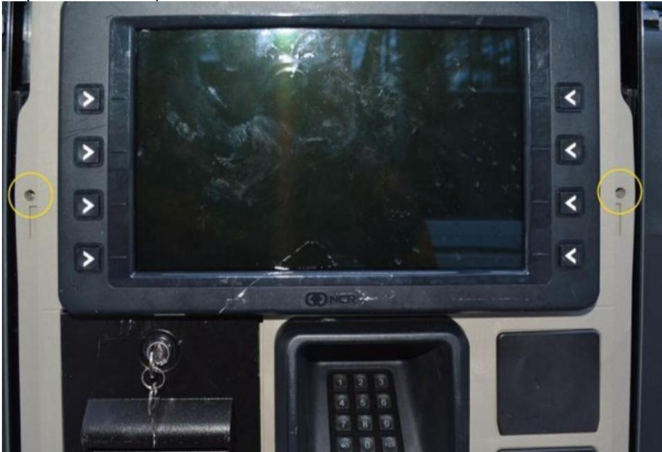
5. Carefully and slowly start to pull out the G7 Helix Standard RFK panel (the slide rails will extend out), until it is partially open as much as possible without stretching the connected cables.
