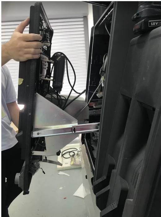
6. On the PPU Board located on the lower part of the G7 Helix Standard RFK panel, mark/label and temporarily unplug the PPU (up to 5 PPUs may be included depending
