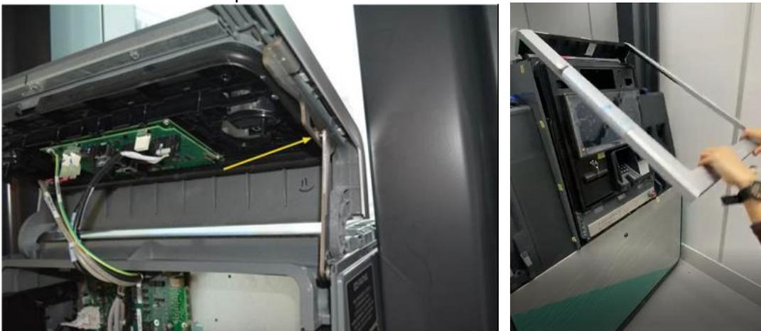
5. Using the provided key for the dispenser, lock the lower metal frame on the Helix dispenser.
