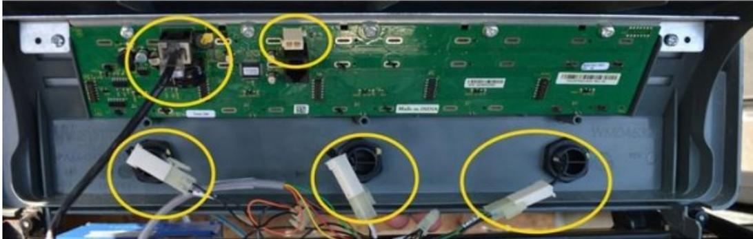
7. On the Helix Customer Display located on the upper part of the G7 Helix Standard RFK panel, mark/label and temporarily unplug the customer display cables and comm speaker (if present) connections and unscrew the grounding wire screw using a T7 Torex driver.
