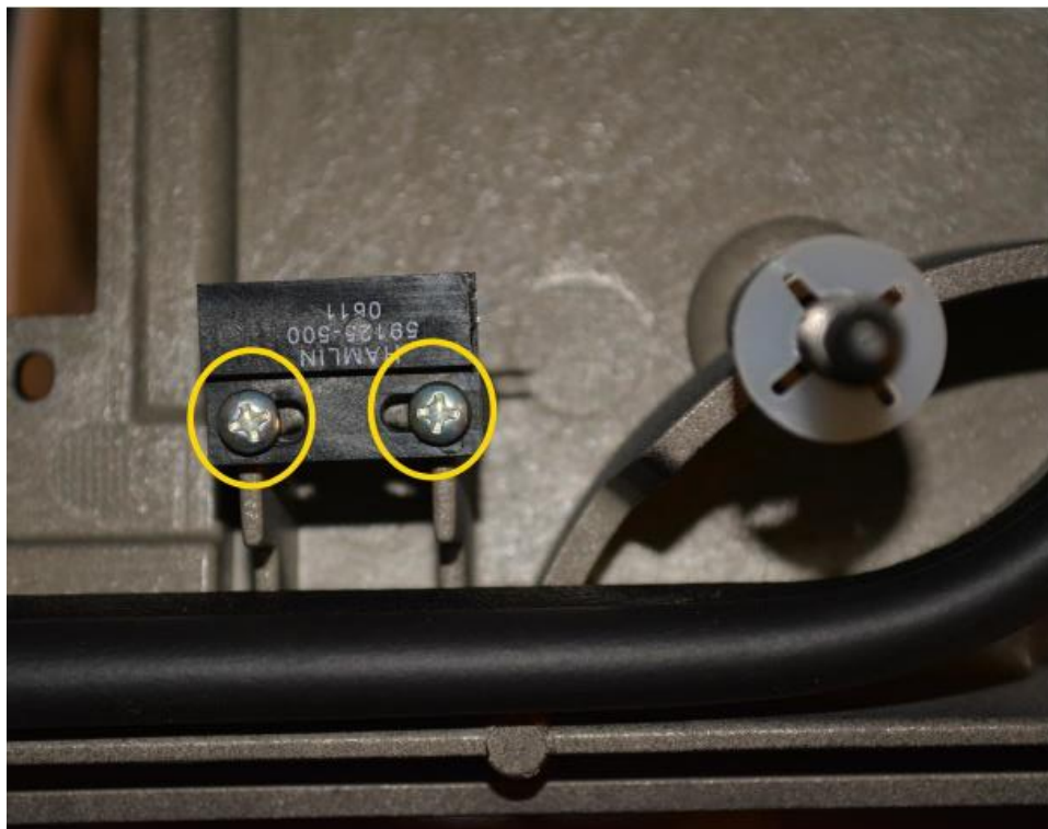
Install with 2 screws per switch
