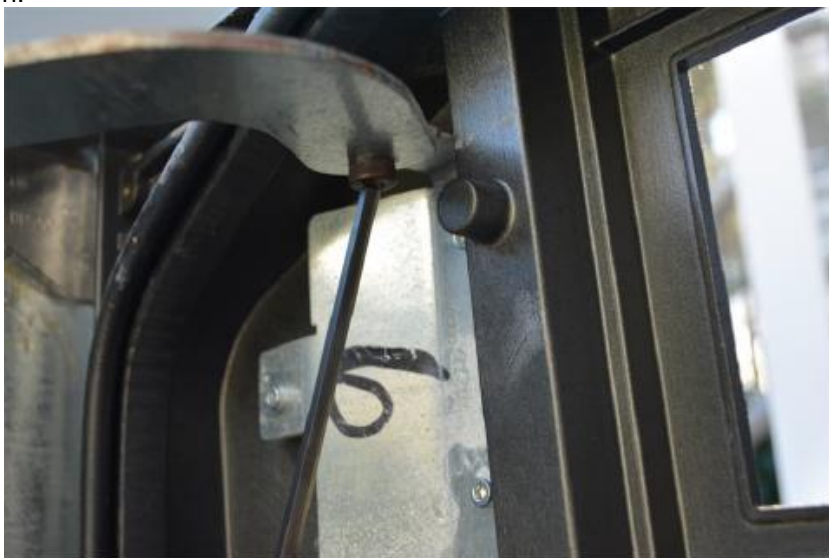
Prop Rod Retaining Hardware
