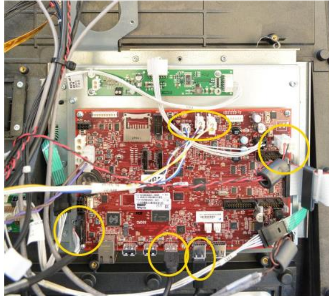
QVGA/VGA (JADE) Cable Removal
