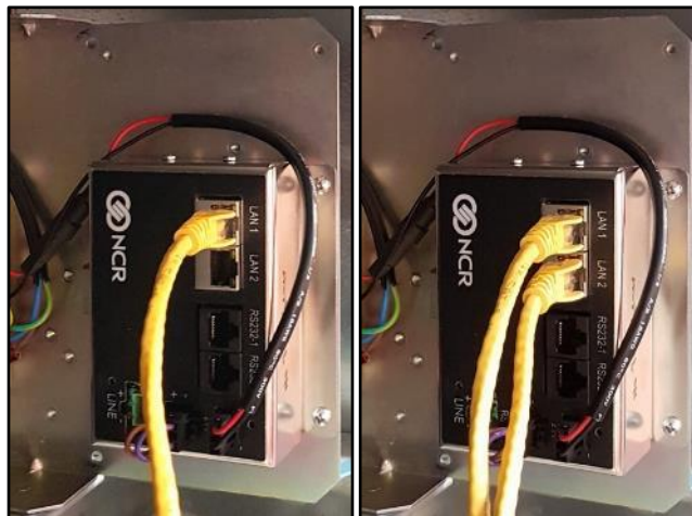
Yellow Cat Cable - Side A (left) and Side A&B (right) connections
