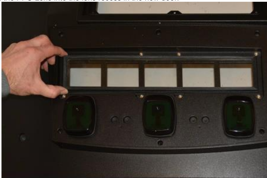
Installing the PPU Lens
