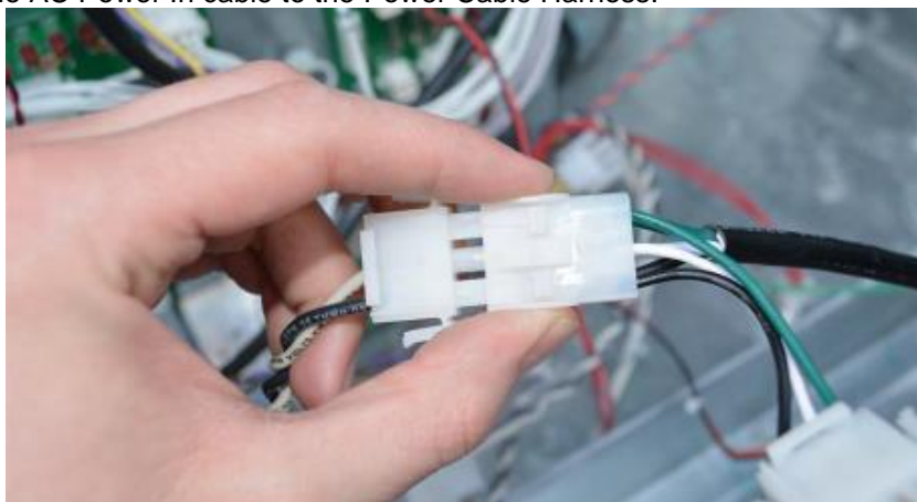
AC Power into Power Cable Harness
