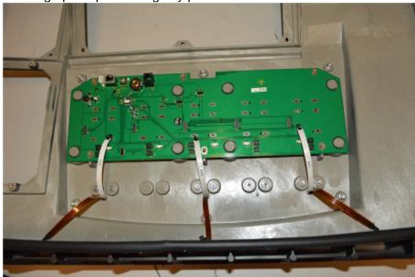
Positioning the PPU Panel
