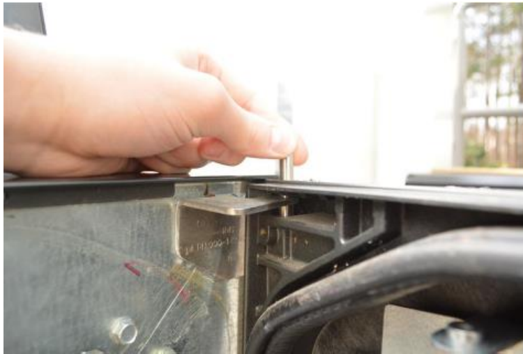
Top Hinge Pin Removal
