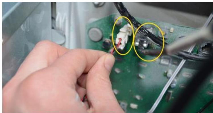
PPU Cables Reinstalled
