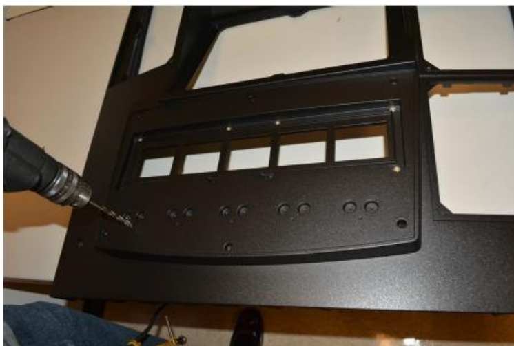
Drilling PPU Flex Holes
