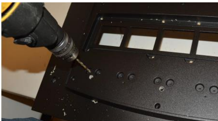
Drilling Bolt Wells
