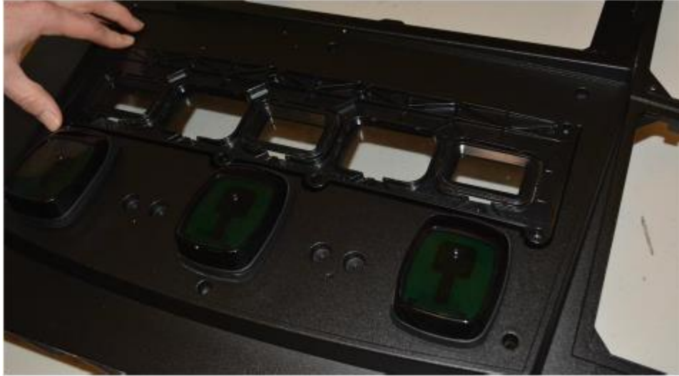
Fitting Retained Lens Cover
