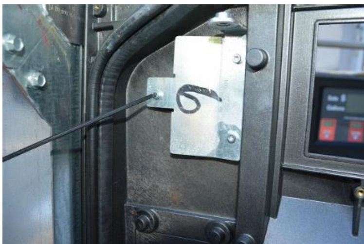
Prop Rod Bracket Removal
