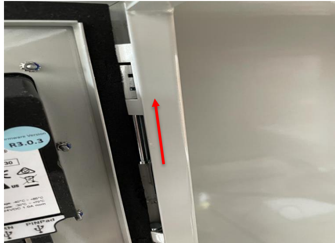
Fig 2.8c – Insert the pin from the bottom to the top.
