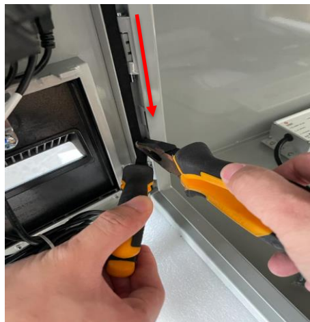
Fig 2.8b – Use a Long nose plier to hold and knock the pin.
