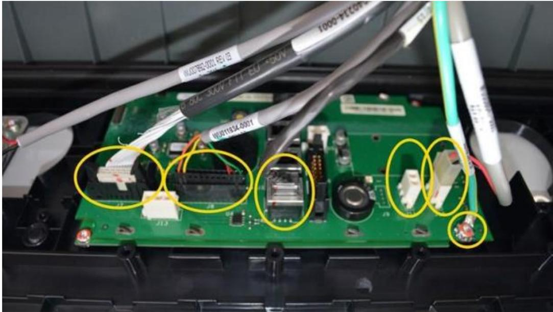
7. Detach the two side tethers using a Philips head screwdriver. Retain the tether attaching screws and washers for later reinstallation, then proceed to section 4.2: Removal of the existing G7 NFC module.
