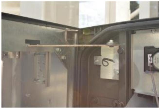
2. Use a Wayne Security Key to screw the two security bolts located on the left-hand side of the dispenser's door face.
