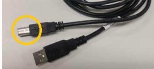
Insert the Type B connector into the “APC-USB” socket on the display (SDC) module (the same socket which had the existing USB cable unplugged in step 3 of section 4.2).
