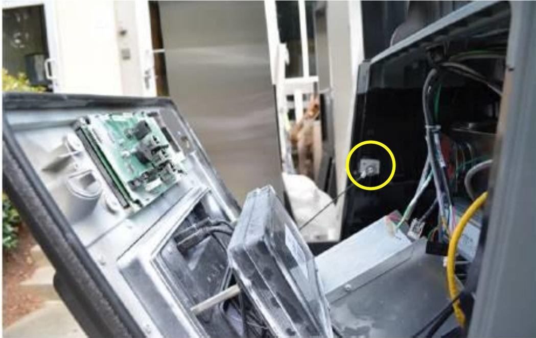
2. Re-plug the customer display cables and comm speaker (if present) connections and re-screw the grounding wire screw using a T7 Torex driver that were marked/labelled and unplugged/unscREWED during the opening of the dispenser (section 4.1.4) on the Helix Customer Display located on the upper part of the G7 Helix Headless RFK panel.
