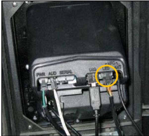
3. Identify the APC module mounted on the rear of the display (SDC) module. From the APC module, unplug the USB cable plugged in the "USB-L" socket. Trace the other end of this same cable and unplug from the "APC-USB" socket on the display (SDC) module. This cable is no longer required and can be discarded.
