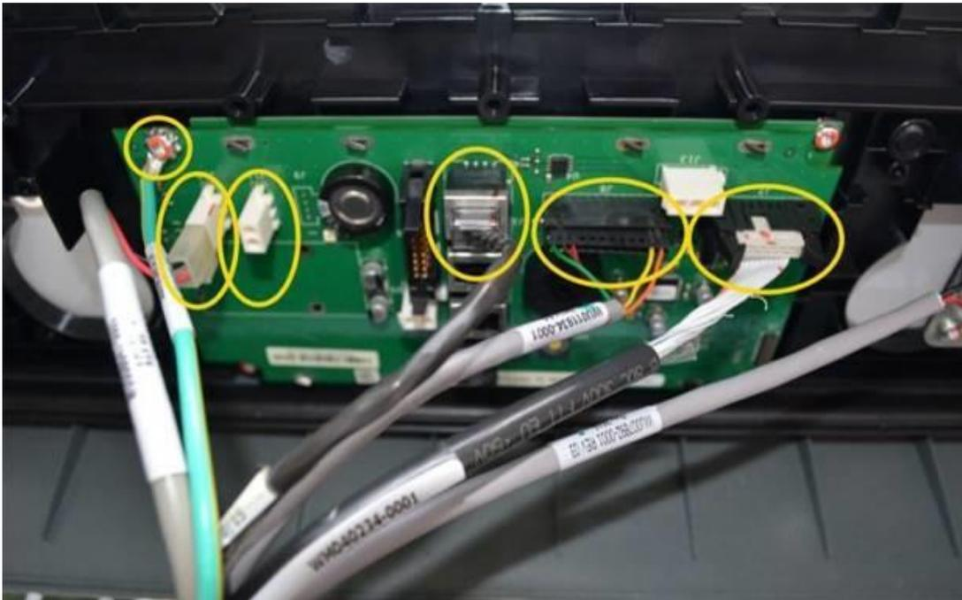
2. On the PPU Board located on the lower part of the G7 Helix Standard RFK panel, re-plug the PPU, Grade Select Button, totalizers (if present), and Call/Intercom Button (if present on PPU panel) connections that were marked/labelled and unplugged during the opening of the dispenser (section 4.1.3).
