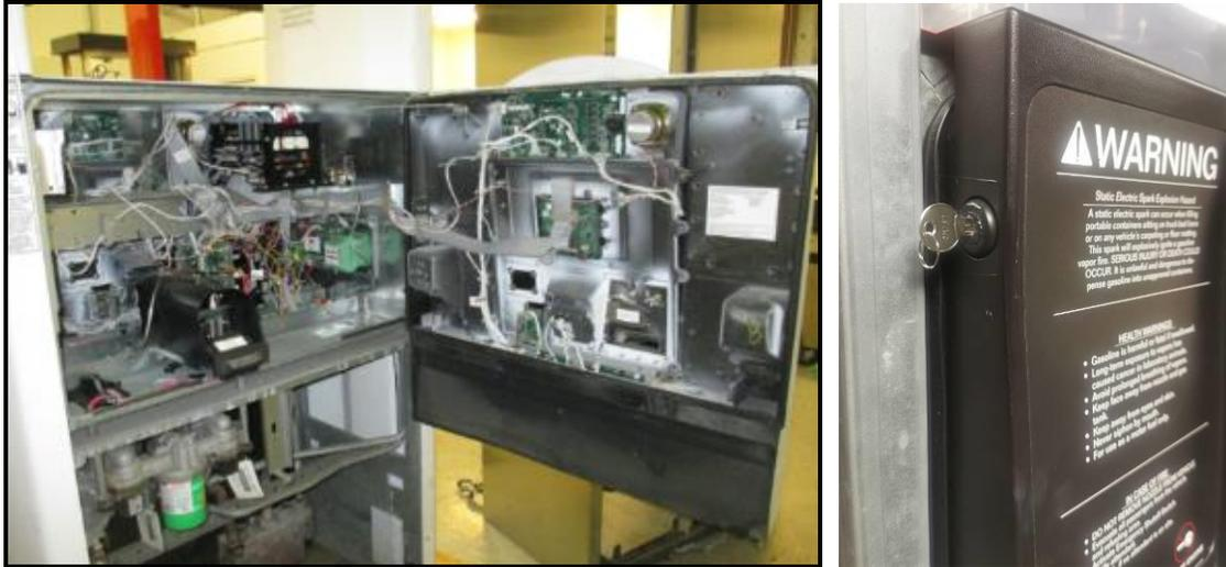
2. Do up the lower door latch located underneath the left-hand side of the Main Dispenser Door.
