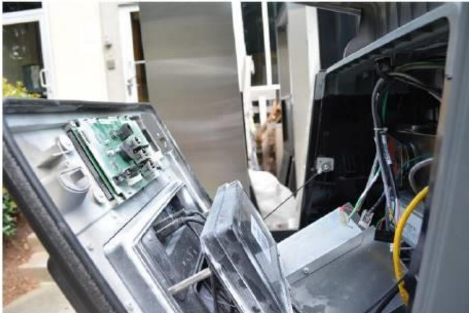
6. On the Helix Customer Display located on the upper part of the G7 Helix Headless RFK panel, mark/label and temporarily unplug the customer display cables and comm
