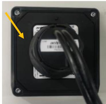
3. Temporarily remove the lock nut that is pre-fitted on the SCC module.
