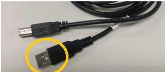
Insert the type A USB connector into the “USB-L” socket on the back of the APC module (the same socket which had the existing USB cable unplugged in step 3 of section 4.2):
