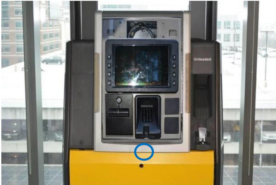
3. Raise the dispenser collar frame and place the Prop Rod in the upper right corner to hold up the dispenser collar frame.
