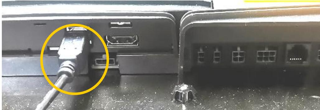
4. Remove the NFC module from the RFK panel by undoing the nut lock by turning it anti-clockwise by hand and pushing the module out and pulling the attached cables out through the same opening. The nut and the NFC module are no longer required and can be discarded.
