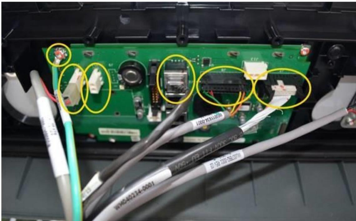
8. Pull out the G7 Helix Standard RFK panel further until the slide rail extends out (as allowed up to the slide rail stop). Then proceed to section 4.2: Removal of the existing G7 NFC module.
