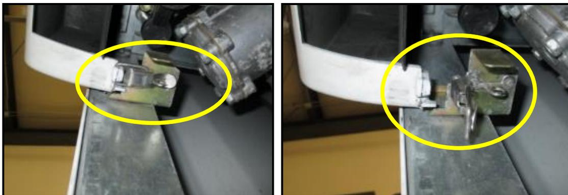
4. Unlock the main dispenser door lock located on the upper left-hand side of the Main Dispenser Door using the "CH 751" key. Open the door until it locks into its fully open position.
