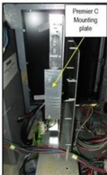
Electronics Cavity after Power Supply is installed
