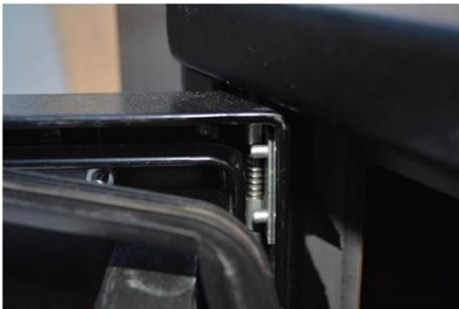
Portion of gasket pulled away revealing door hinge
