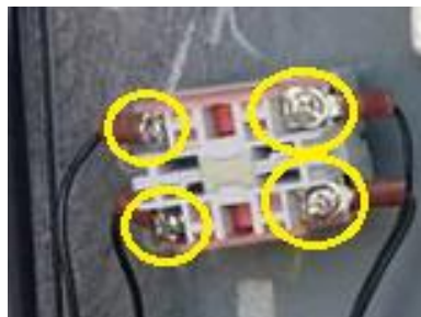
Fig 4.9e – Screw the previously marked wiring back on to the Emergency stop button.
