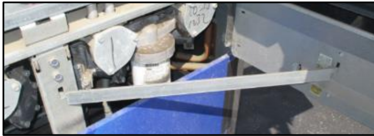
Fig 2.6 c – Door prop inserted in prop position
