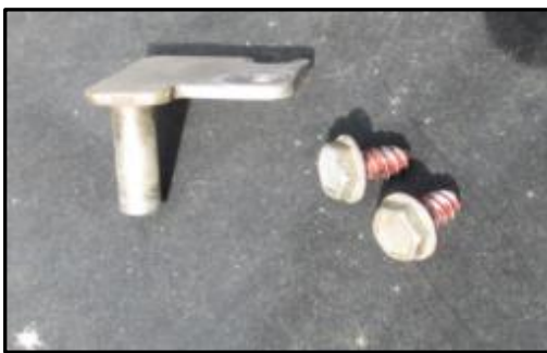
Fig 2.9 d – Upper hinge pin and screws
