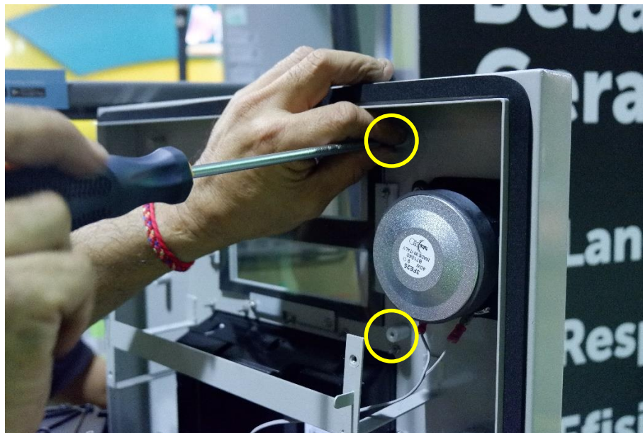
Fig 4.9a - Use a Philips screw driver to remove the screw.
