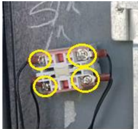
Fig 2.3f –Remove the wiring from the Emergency stop button terminals and mark for later reconnection to the same retained Emergency stop button
