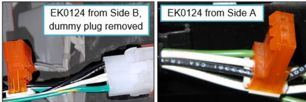
Fig 4.5 – Connections for EK0124's – Side-B
