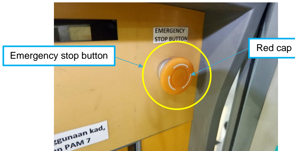
Fig 2.3g – Remove the red cap by turning it anti-clockwise.
