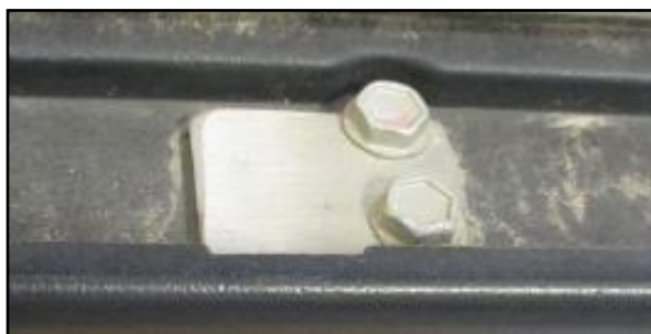
Fig 4.7 d – Upper hinge pin after tightened.
