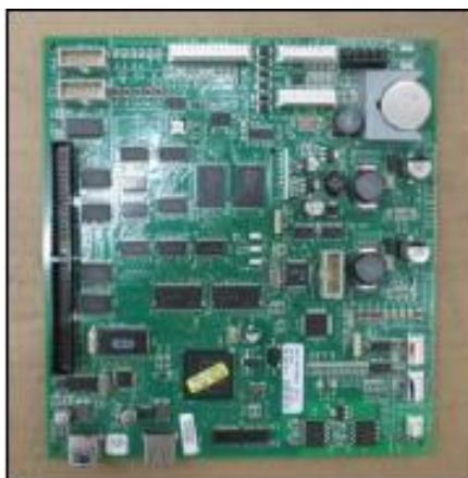
Fig 2.12b – CRIND Control Node after removal
