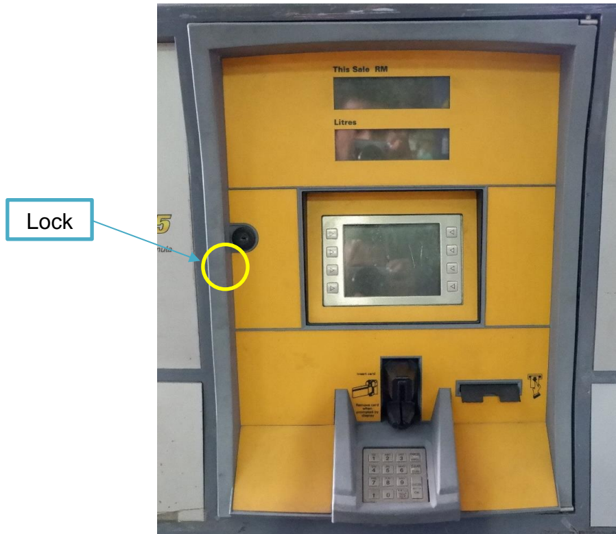
Fig 2.1a – Access door and lock location for Encore 300 or 500
