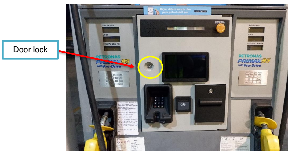
Fig 4.22b – Completed OPT installation for the Encore 300Q or 500Q
