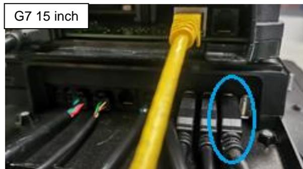
39. Plug EK0117 into the "PRINTER PWR" socket on the G7 or the G7 15 inch SDC:
