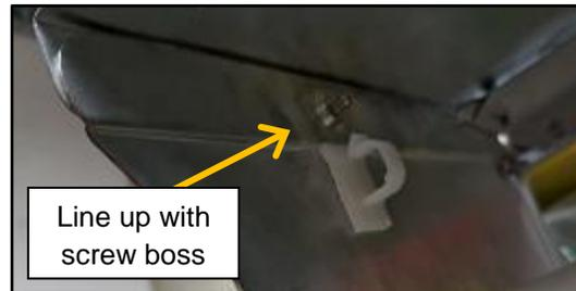
24. Attach 1X MN0046 self-adhesive Cable Clip to the top back center of the Lid MP0533.
