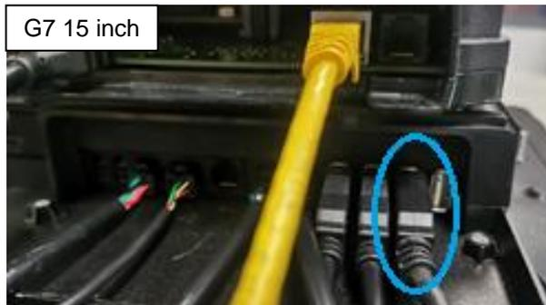
8. If you wish, trace the printer's Power Cable to its source, unplug that end and then discard the cable – it will not be re-used.
