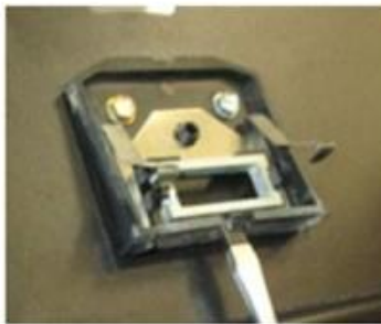
Fig 1.3c – Flathead screwdriver pushing in on lock tab
