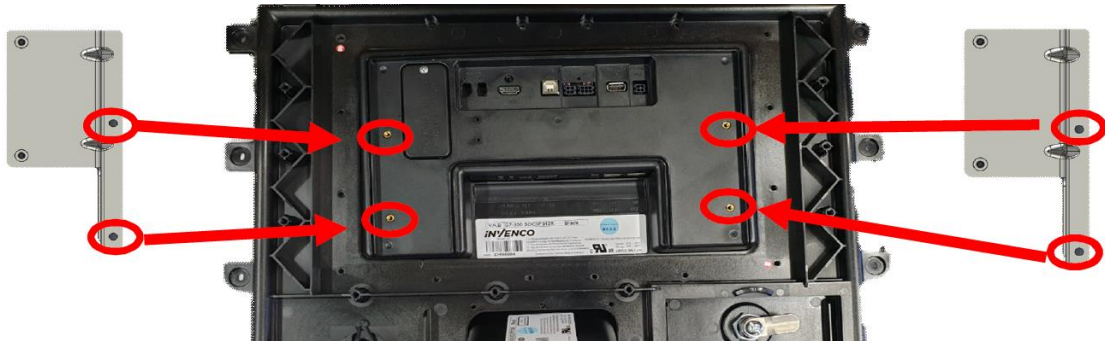
Removing the screws that hold the APC mounting brackets in place
