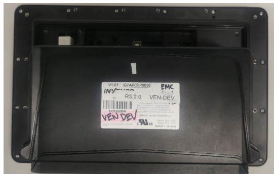
Rear View – note the APC module is mounted on the G7 SDC module
