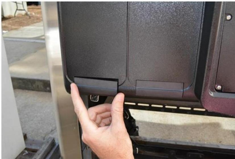
2. Remove the adhesive liner on the Aluminum Blank **MP0962** and place into the boot recess adhesive side towards the door. Attach with two Phillips screws **MS0238** at the top and two machine screws in the middle **MS0239**. Install the blanks where a nozzle boot will **not** be installed.
