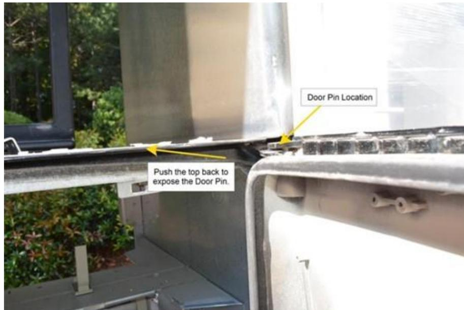
5. With the door fully open and supported at the bottom, use a pair of needle nosed pliers to firmly grasp the hinge pin and pull upwards to remove it. Discard the pin.
