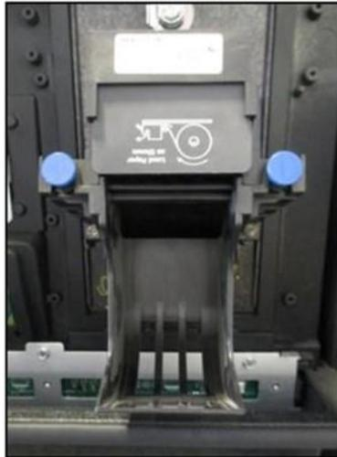
*Fig 1.13 – Screws holding down printer bracket*
