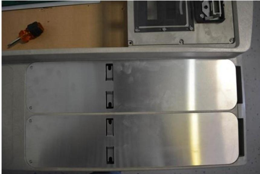
3. Install the top boot bracket aluminum blank **MP0964** to fill any gaps in the boot recess where the boot will be installed. Attach with two Phillips screws **MS0238**.
