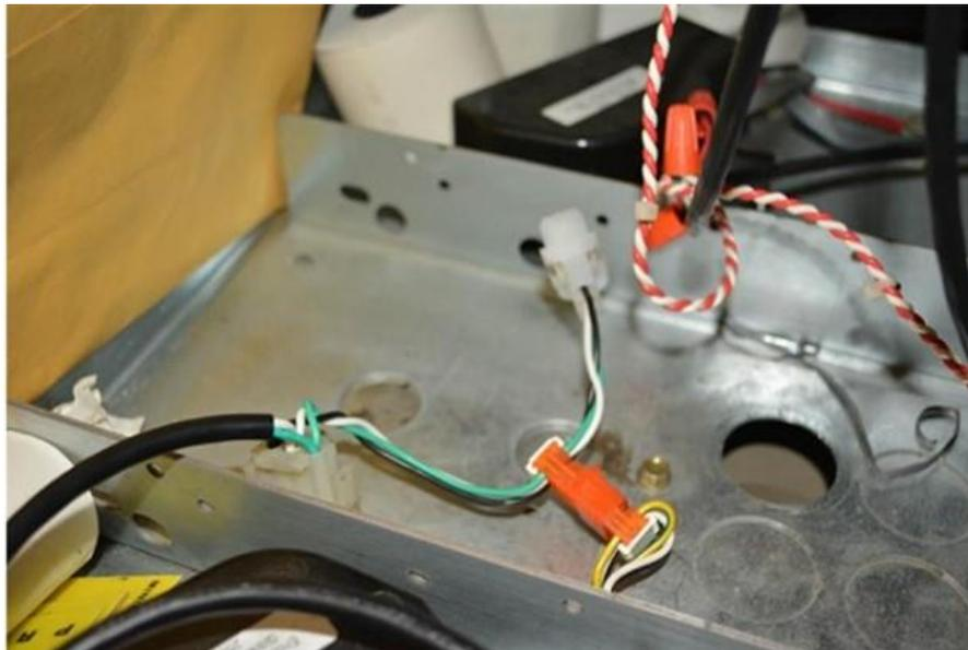
*Wiring in the Power Supply to the Pump Power Distributor for Second Installed (B Side) PSU*
