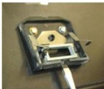
*Fig 1.3c – Flathead screwdriver pushing in on lock tab*
