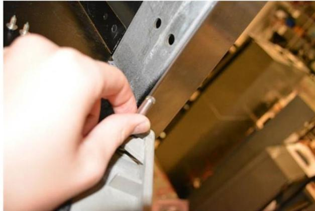
3. Install the weather shield (previously retained) to the modular door with five screw bolts (previously retained) with the prop bar storage hooks facing towards you.
