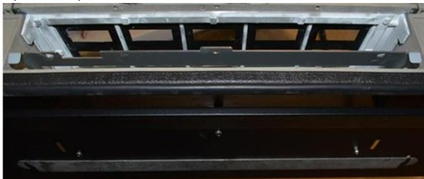
**Note:** Verify the correct orientation and locations of the PPU screens when installing the PPU Bracket.
