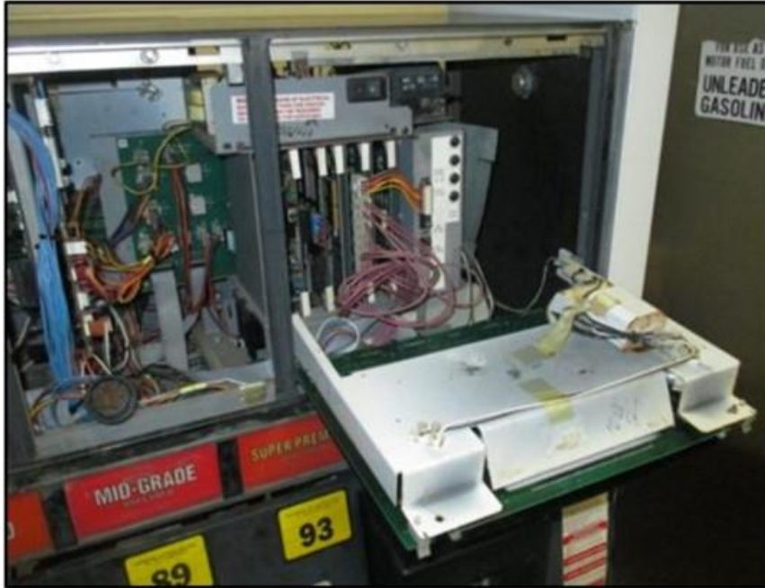
Money/Volume Display Assembly in fully forward position
