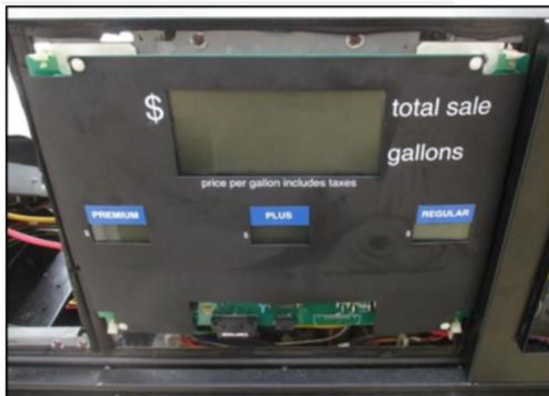
Money/Volume Display assembly re-fastened to Dispenser Frame
