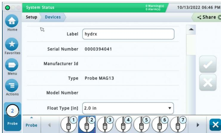
Figure 2. Example Probe Setup Screen
