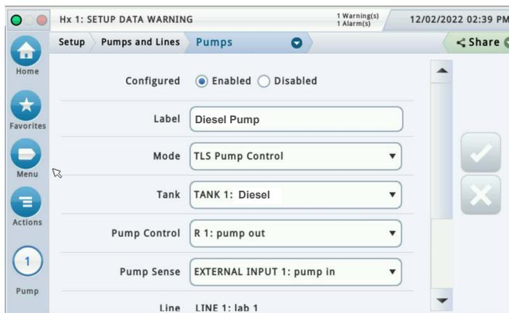
Figure 9. Example Pumps Setup Screen
