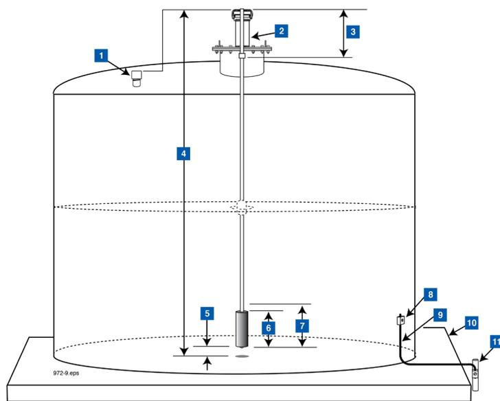
1. Insertion measuring point for 2" (5.08cm) pipe cap installations (top of pipe cap to tank bottom)
